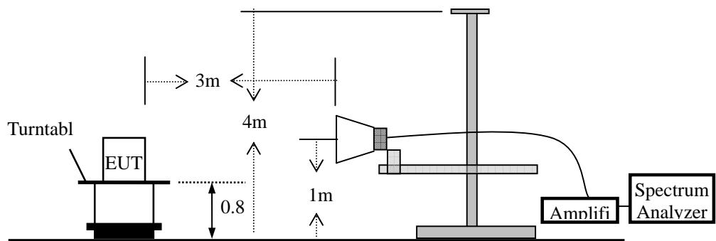
**Substituted Method Test Set-UP**
