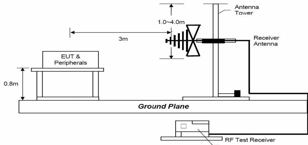
**Radiated Emission Test Set-Up, Frequency above 1GHz**
