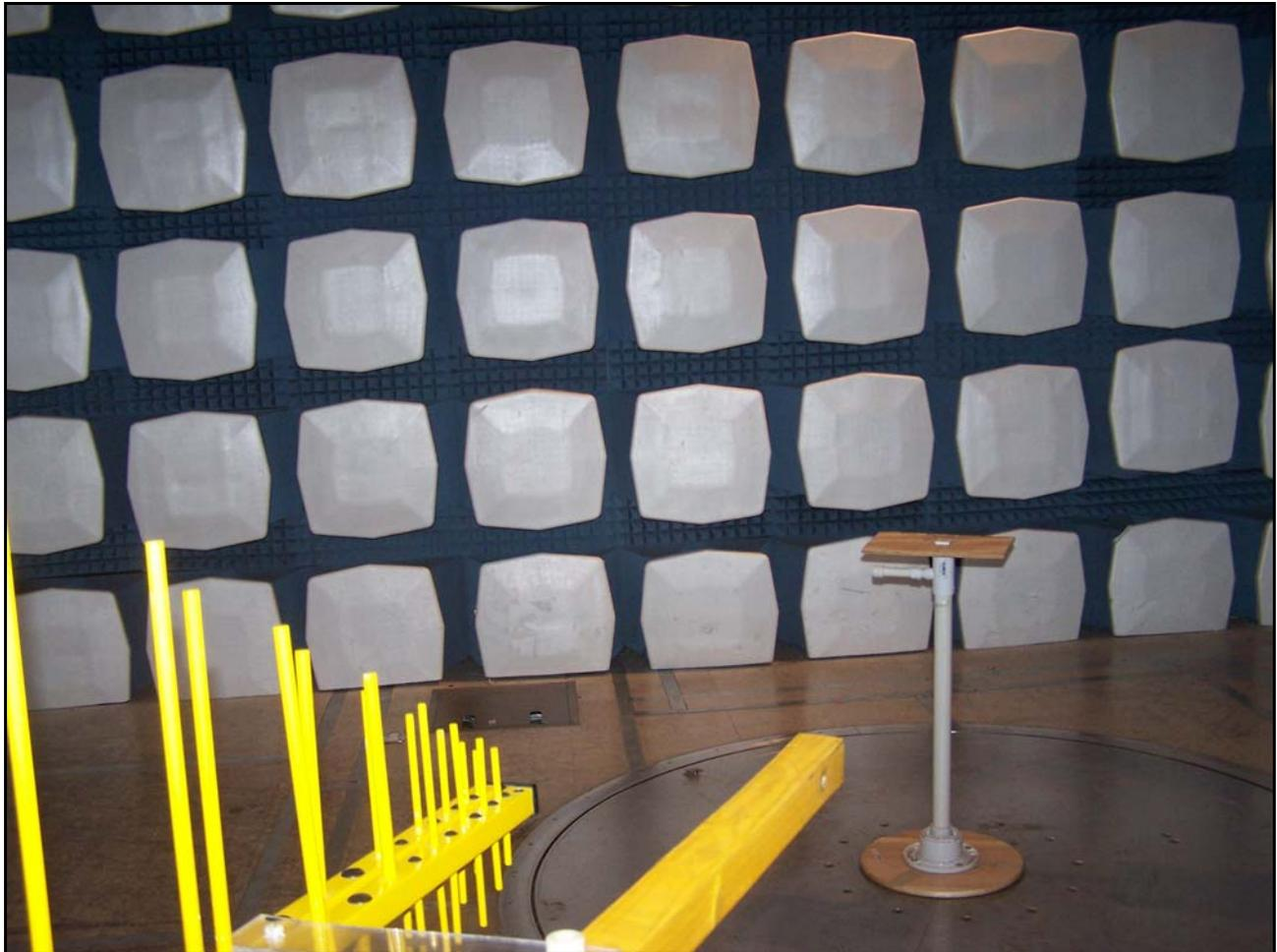
**Photograph 5. Radiated Emissions Below 960 MHz, Test Setup**
