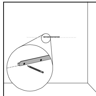
If you're installing a SMART Board 685/SBD685 or 690/SBD690 interactive whiteboard, space your wall-mounting brackets 4" (10.2 cm) or 6" (15.3 cm) apart respectively, and then mark the location of the ten mounting holes on the wall.
