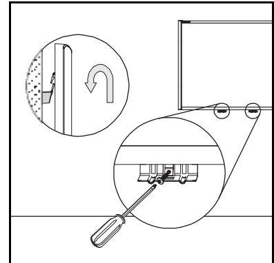
4. Position the pen tray in line with the two L-shaped metal brackets, and then slide it toward the wall until it rests snugly against the bottom frame of your interactive whiteboard.
