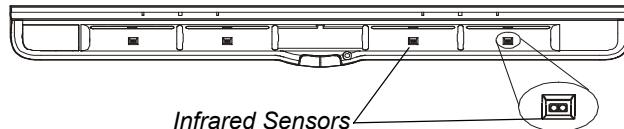
To clean a sensor, moisten a cotton swab with a household glass cleaner, such as Windex, and then carefully clean the infrared transmitter and receiver.
