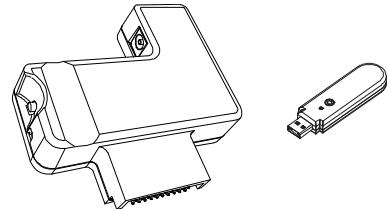
The wireless Bluetooth connection expansion module plugs into the controller module on the back of your interactive whiteboard, and the Bluetooth-to-USB converter plugs into your computer's USB receptacle. To ensure a secure connection, the SMART Board interactive whiteboard expansion module and USB converter support 128-bit encryption.
