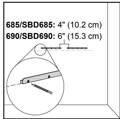
3. Use the Phillips No. 2 screwdriver to secure an included self-tapping wall anchor at each mark.
