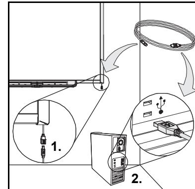
2. Connect the other end of the USB cable to a USB receptacle on your computer.
