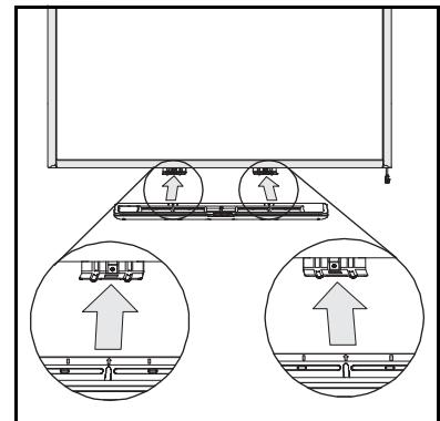
5. Route the modular I<sup>2</sup>C cable through the cable management channel under the lower-right end of the pen tray, and then insert its connector into receptacle 1.
