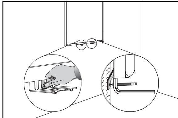
2. Remove your interactive whiteboard from the wall, and then use the screwdriver to secure a self-tapping wall anchor at each mark.
