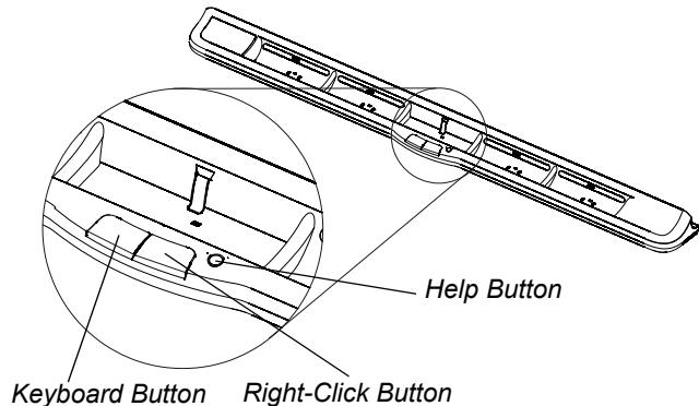
In either mode, you can customize the buttons using SMART product drivers to provide several other functions, including printing, changing pages, launching applications and capturing the screen. Pressing both buttons simultaneously starts the orientation process.
