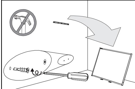
3. With the help of another person, hang your interactive whiteboard back on the wall-mounting bracket, and then secure the L-shaped metal brackets to the wall anchors with the included screws, as illustrated.
