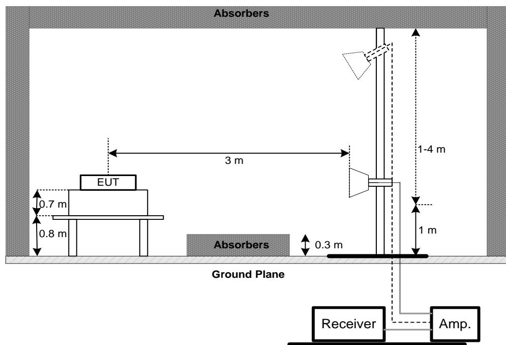
(C) For Radiated Emissions Below 30MHz
