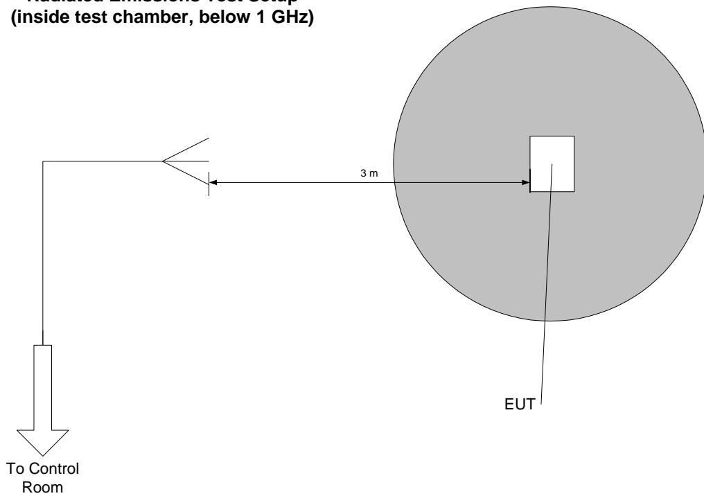
**Radiated Emissions Test Setup
