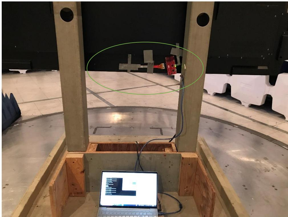
During Radiated Emissions testing, the BLE module is configured to constantly transmit on the Low, Mid or High channel using the provided SMART Tech laptop with the ATM RF Test Tool.
