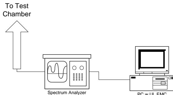
**Radiated Emissions Test Setup
