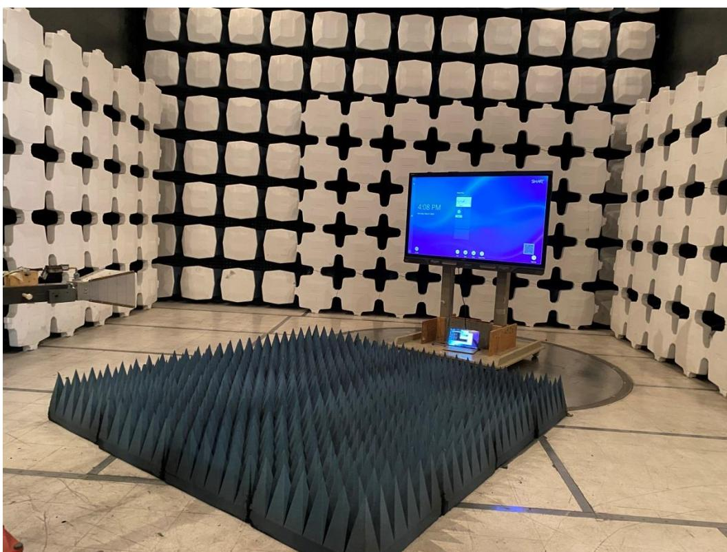
**Photo of Radiated Emissions test setup: 18-26.5GHz**
