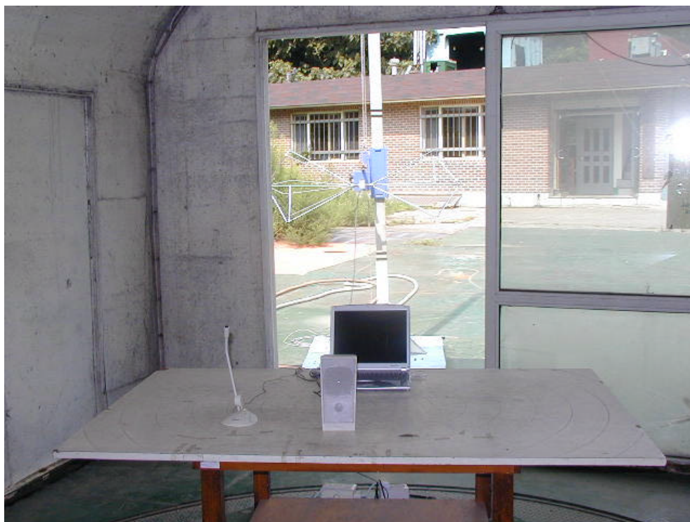
RADIATED EMISSION SETUP PHOTOGRAPH - FRONT VIEW ( 30 - 300 MHz )
