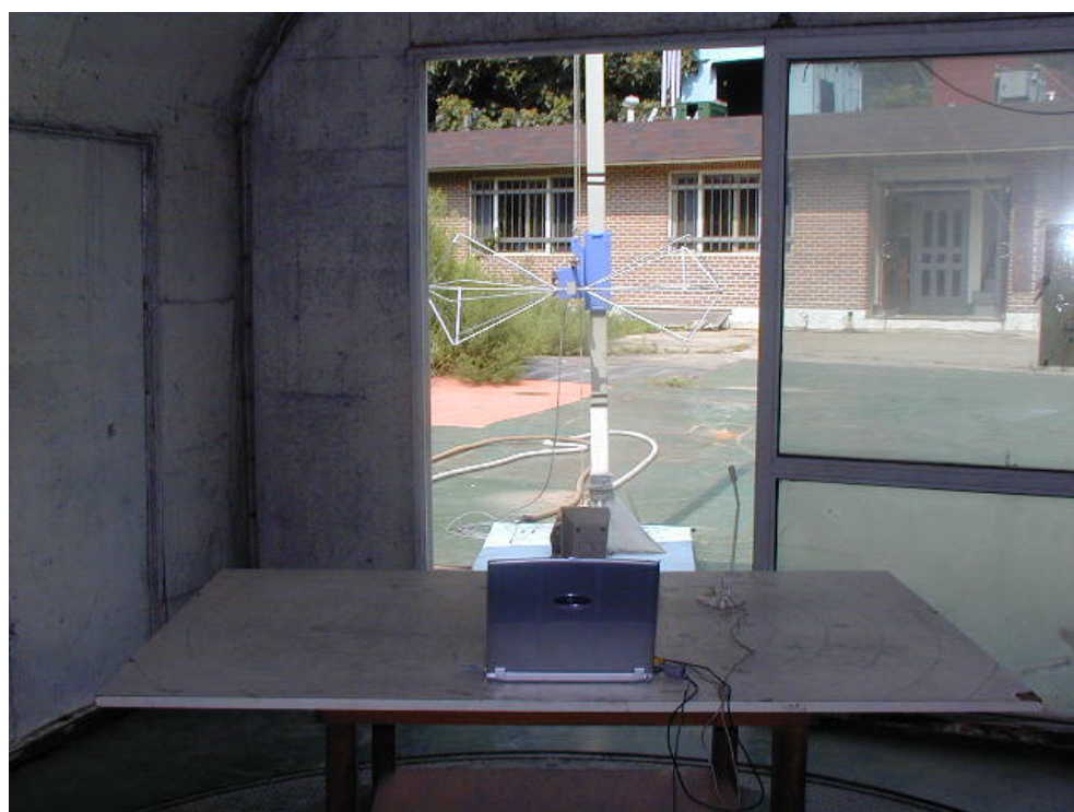
RADIATED EMISSION SETUP PHOTOGRAPH - REAR VIEW ( 30 - 300 MHz )
