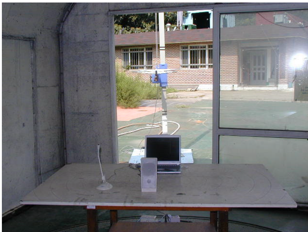
RADIATED EMISSION SETUP PHOTOGRAPH - FRONT VIEW ( 300- 1000 MHz )
