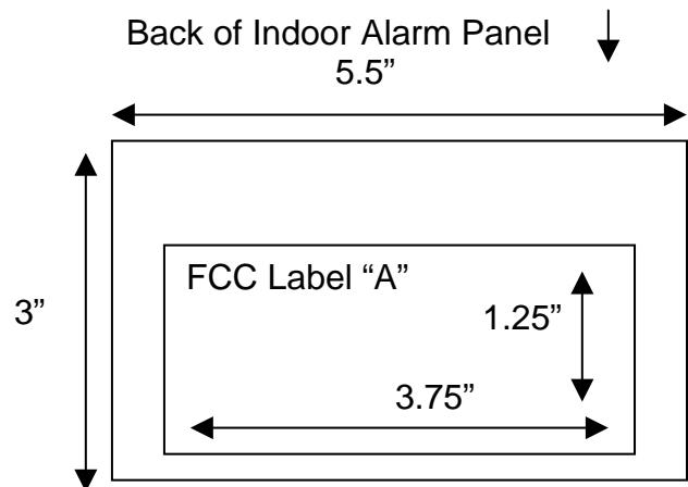
Label is 1.25" x 3.75" placed onto the back of the Indoor Panel
