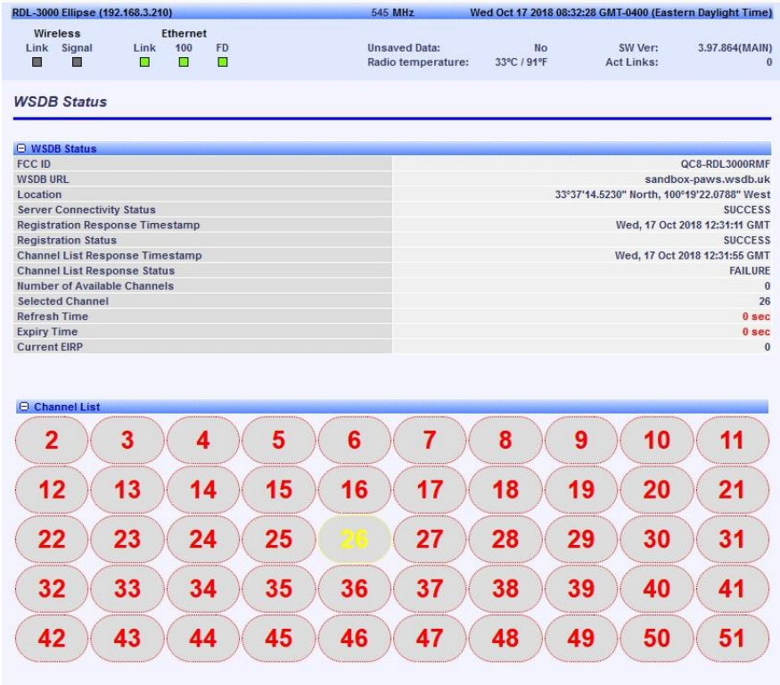
Figure 8.14-2: Data log of unsuccessful registration with restricted antenna height empty channel list
