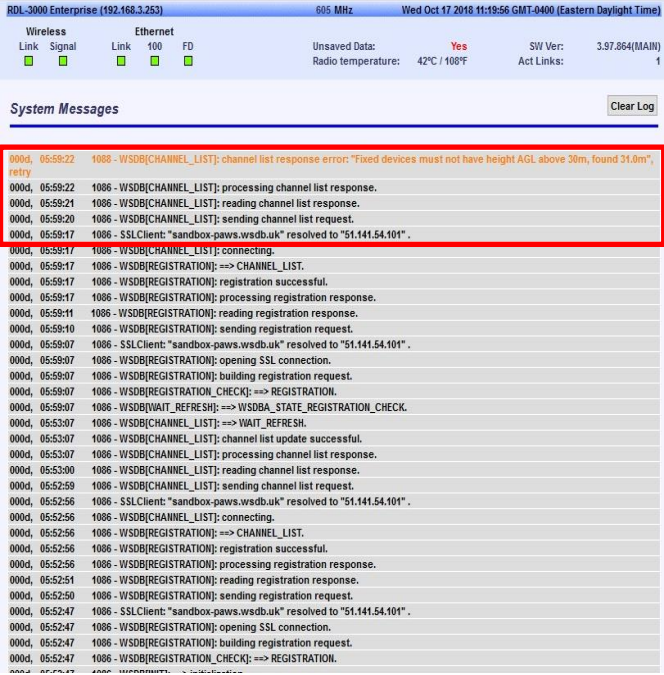
Figure 8.14-3: Data log of unsuccessful registration with restricted antenna height of Subscriber device
