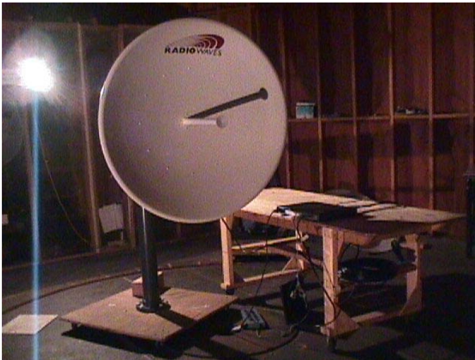
Photo #1: Radiated Emissions Measurements at 3m Distance with Radiowave Antenna Model SP4-5.2NS, Gain: 34.8 dBi (maximum gain within its family)
