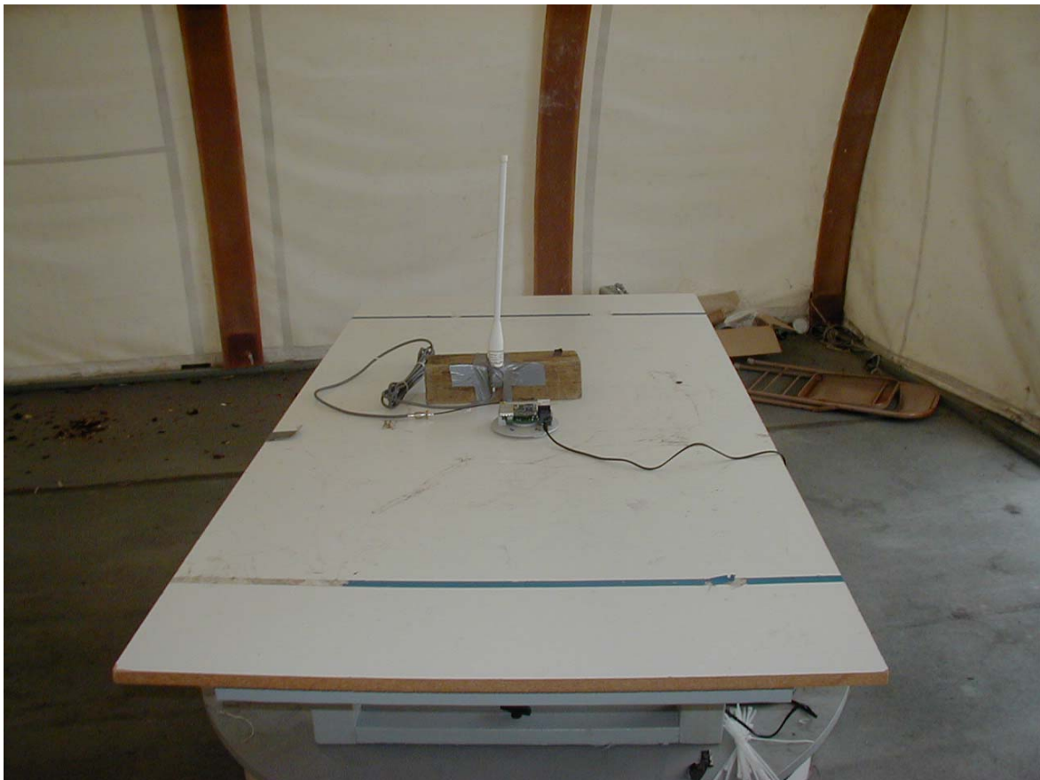
Radiated Emissions in Restricted bands with “omni” antenna
