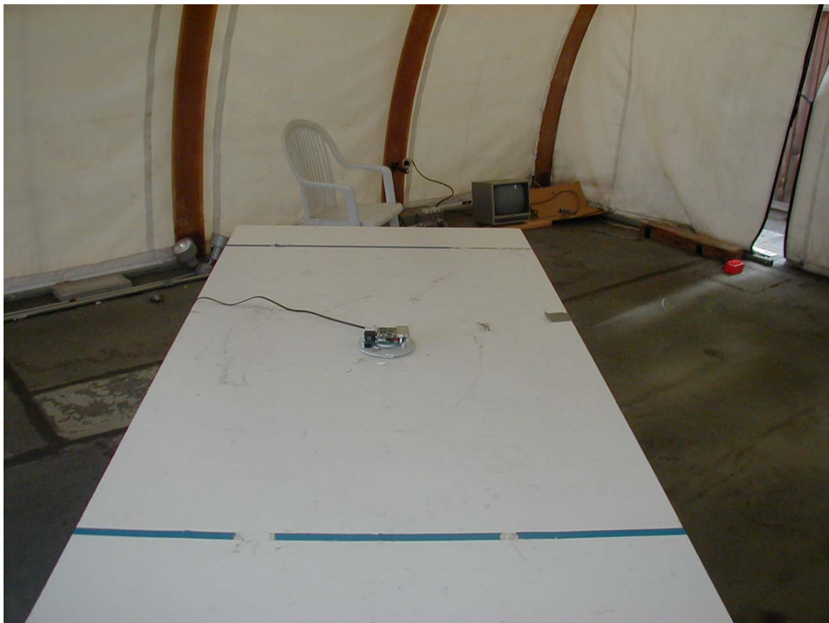
Radiated Emissions in Restricted bands with “helical” antenna
