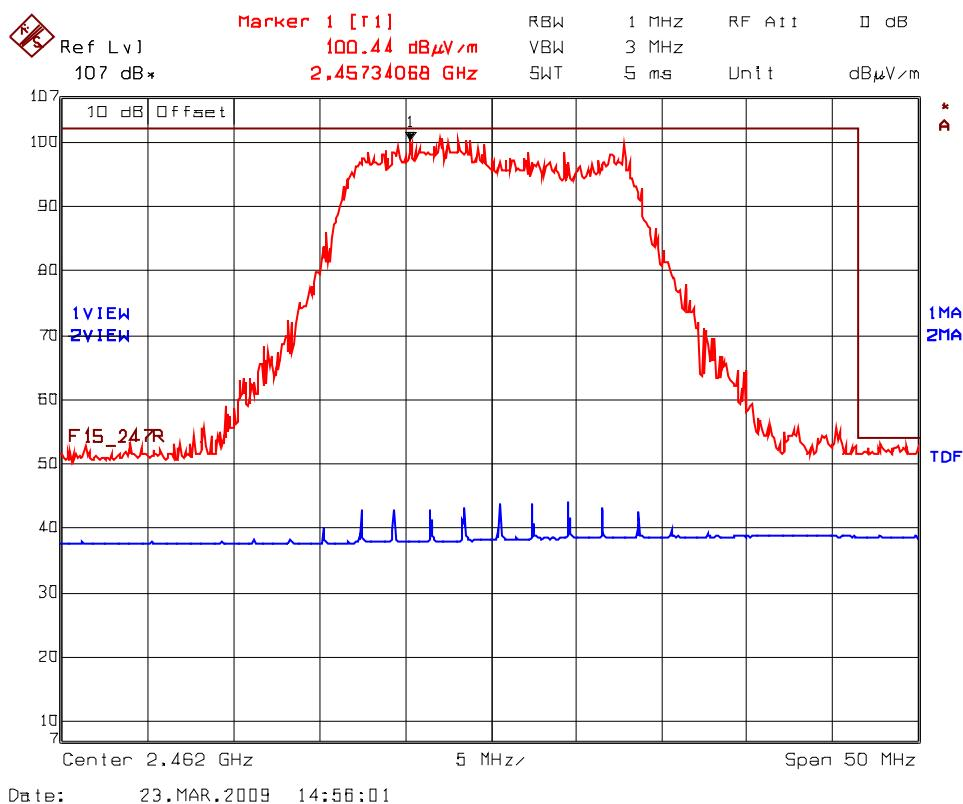
**Plot 5.8.5.1.8** Band-Edge RF Radiated Emissions @ 3 m
