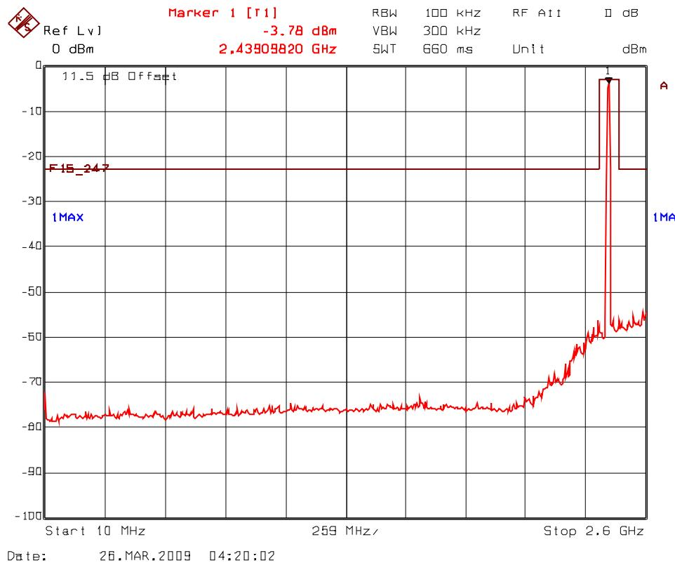
**Plot 5.7.5.2.2(ii) Spurious RF Conducted Emissions, 802.11b Mode**
