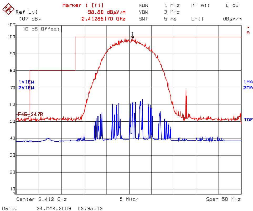
**Plot 5.8.5.1.3** Band-Edge RF Radiated Emissions @ 3 m
