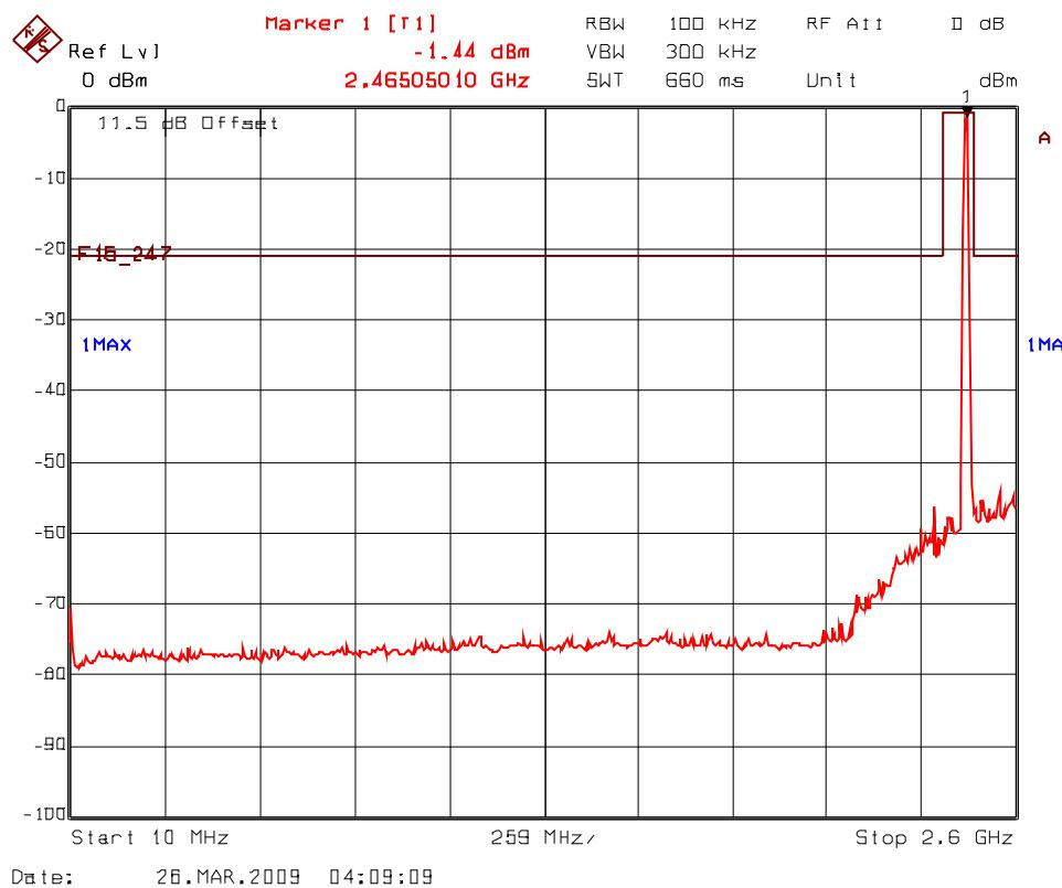
**Plot 5.7.5.2.3(ii) Spurious RF Conducted Emissions, 802.11b Mode**
