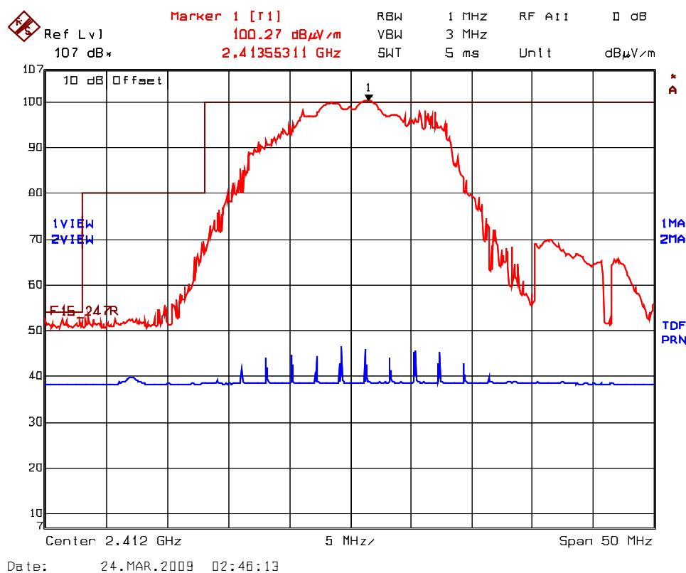
**Plot 5.8.5.1.7** Band-Edge RF Radiated Emissions @ 3 m
