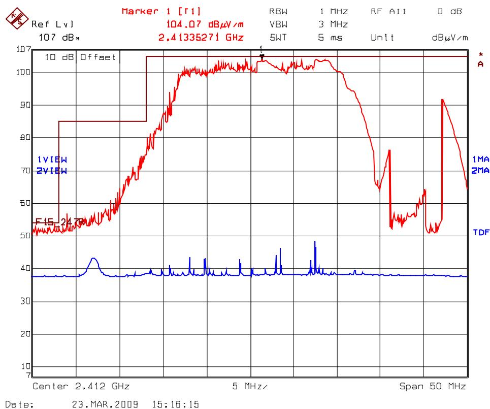
**Plot 5.8.5.1.6** Band-Edge RF Radiated Emissions @ 3 m
