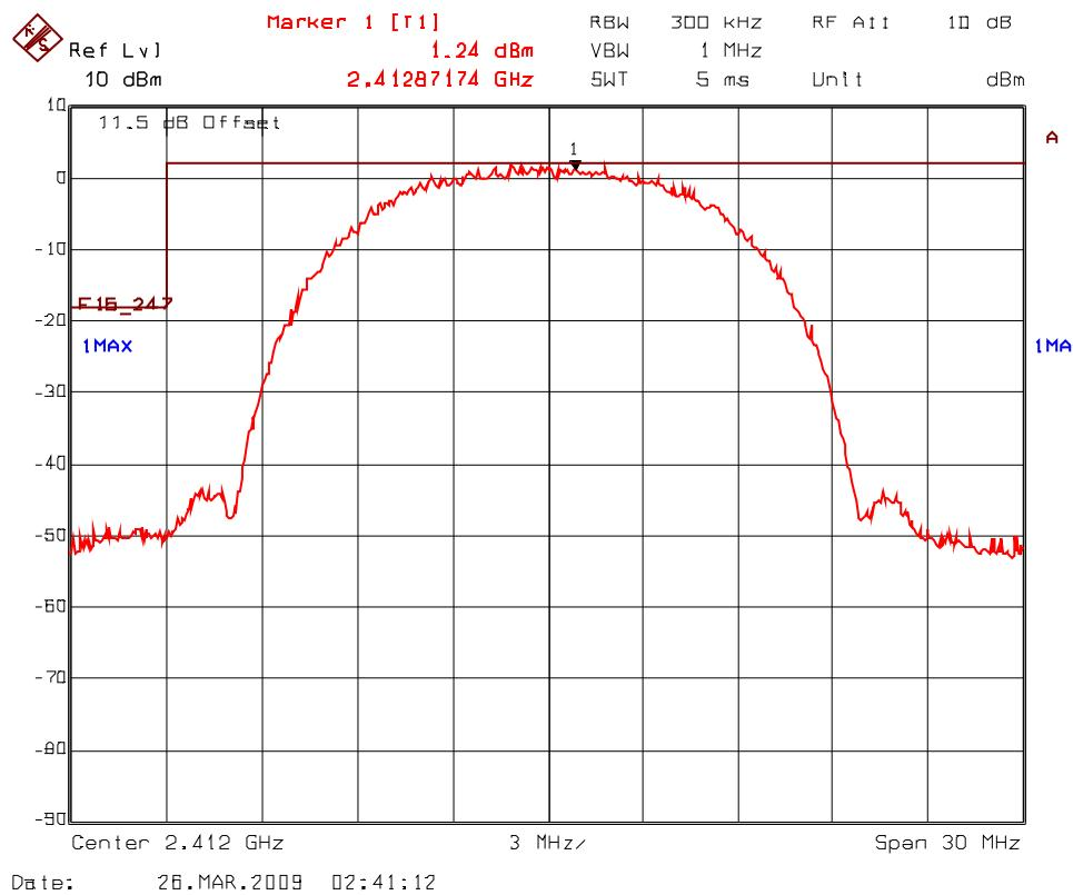
**Plot 5.7.5.1.2 Band-Edge RF Conducted Emissions, 802.11b Mode
