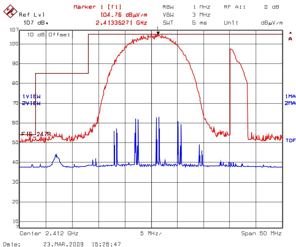
**Plot 5.8.5.1.2** Band-Edge RF Radiated Emissions @ 3 m
