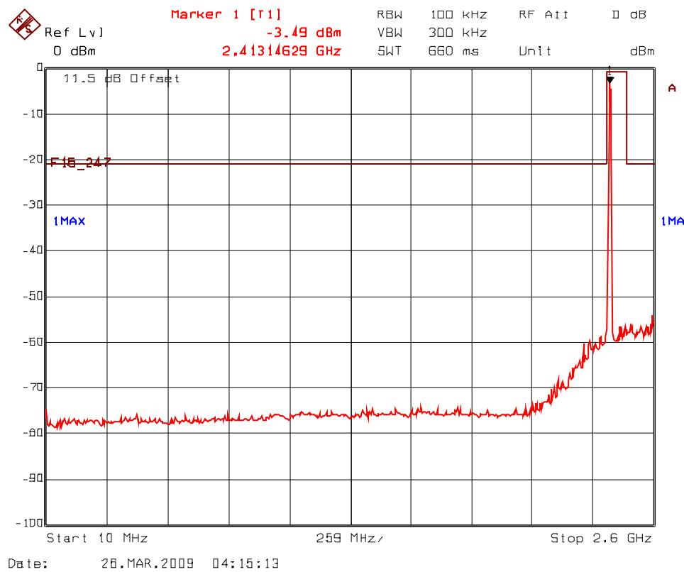
**Plot 5.7.5.2.1(ii) Spurious RF Conducted Emissions, 802.11b Mode**
