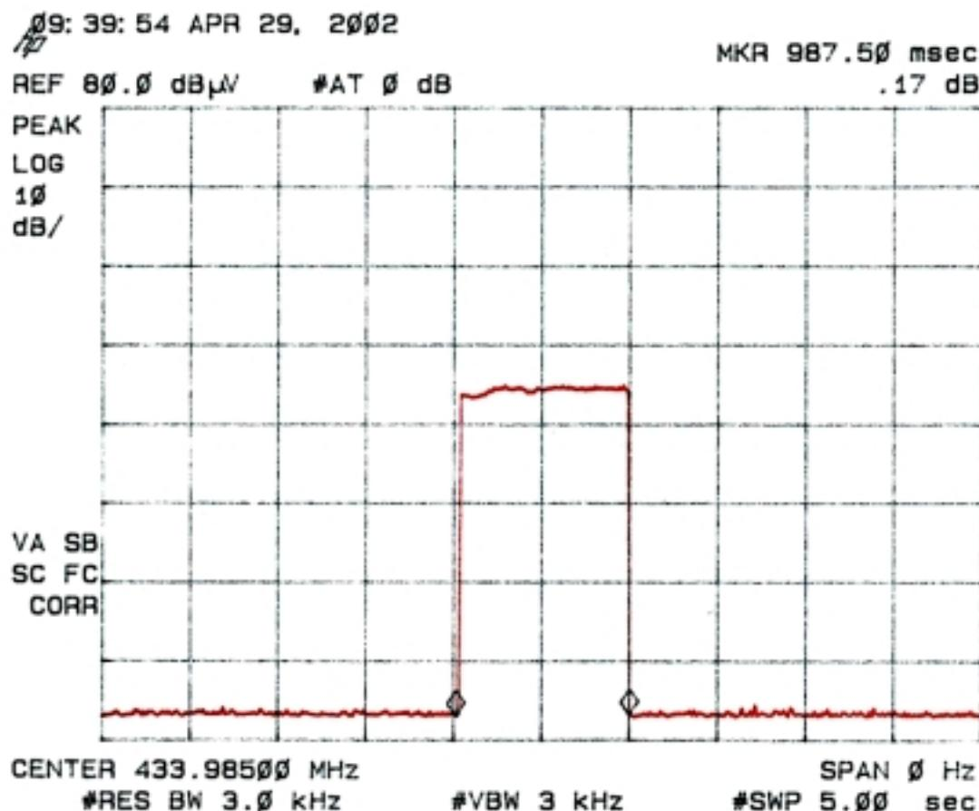
『**Remark:** The devices (Radio Frequency Remote Control Thermostat/Transmitter Unit, EUT) operation the duration of each transmission is not greater than one second and the silent period between duration of the transmission but in no case less than 10 seconds, Compliance with §15.231 (e)』
