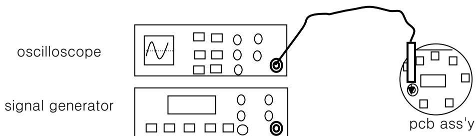
signal generator Rf board output level -85dbm
