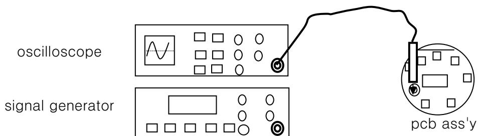
signal generator Rf board output level -85dbm
