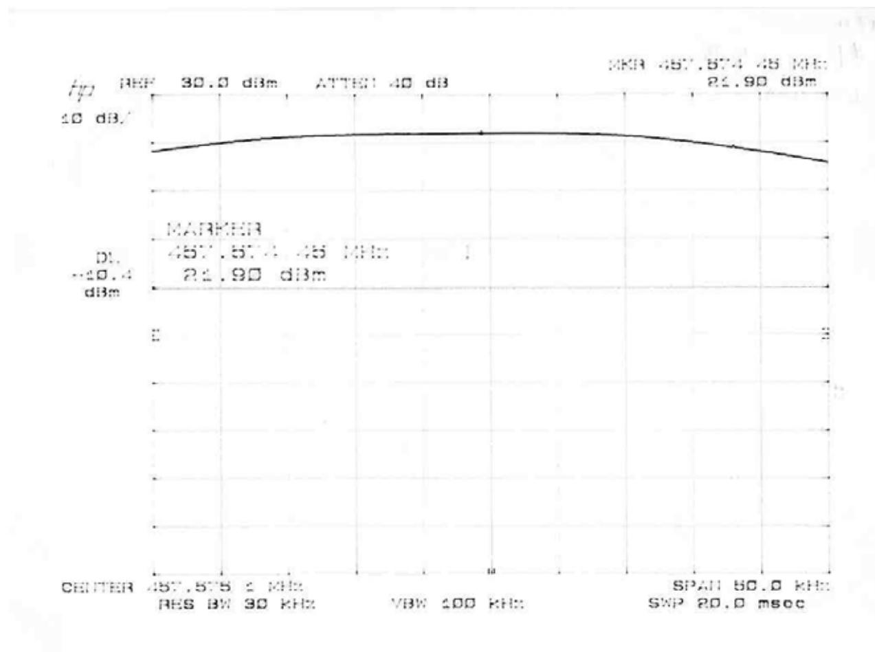
C-factor : 5dB ; (C-factor = Attenuator + Cable Loss)
