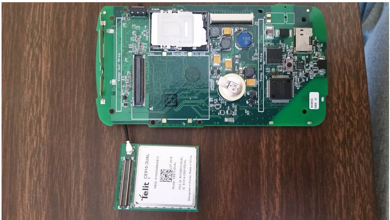
Figure 6: PCBA - Top with Telit Module
