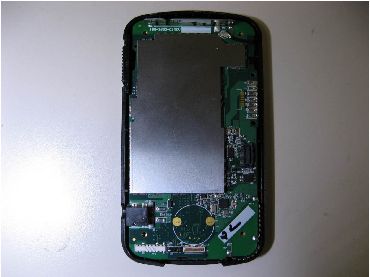
Figure 1: PCBA – Bottom view with shield
