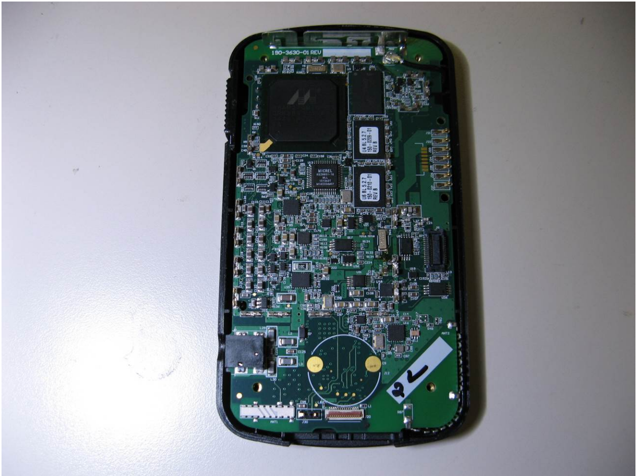
Figure 2: PCBA – Bottom view without shield
