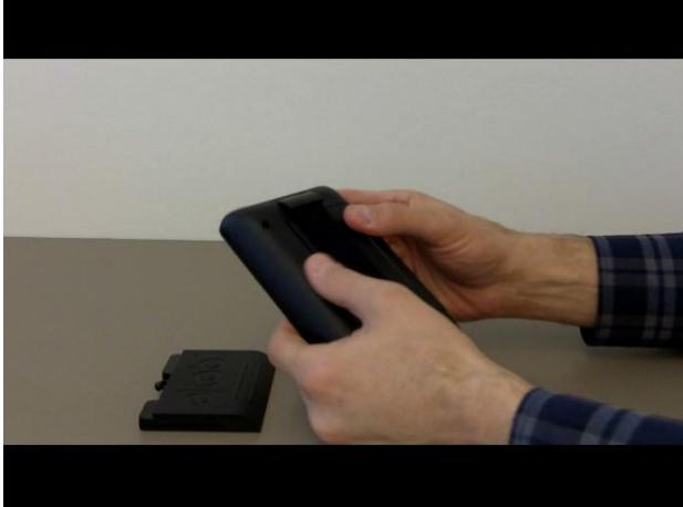
2. While pulling down the release latch, slide the battery out of the device.
