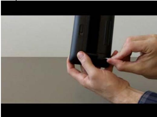
3. Hold the power button down until the device turns on; then release the paper clip.
