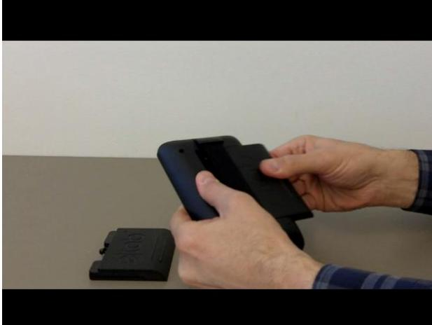
3. Slide a fully charged battery into the battery slot until the latch clicks.
