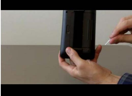
2. Insert the end of the paper clip into the small hole in the back of the device; hold until you feel the power button click.
