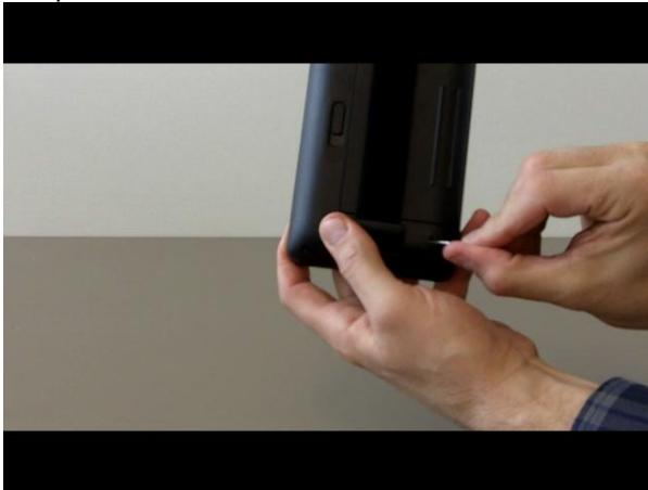
3. Hold the power button down until the device turns off; then release the paper clip.
