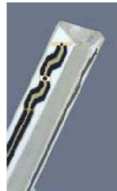
Figure 2.3 Probe Thick-Film Technique
