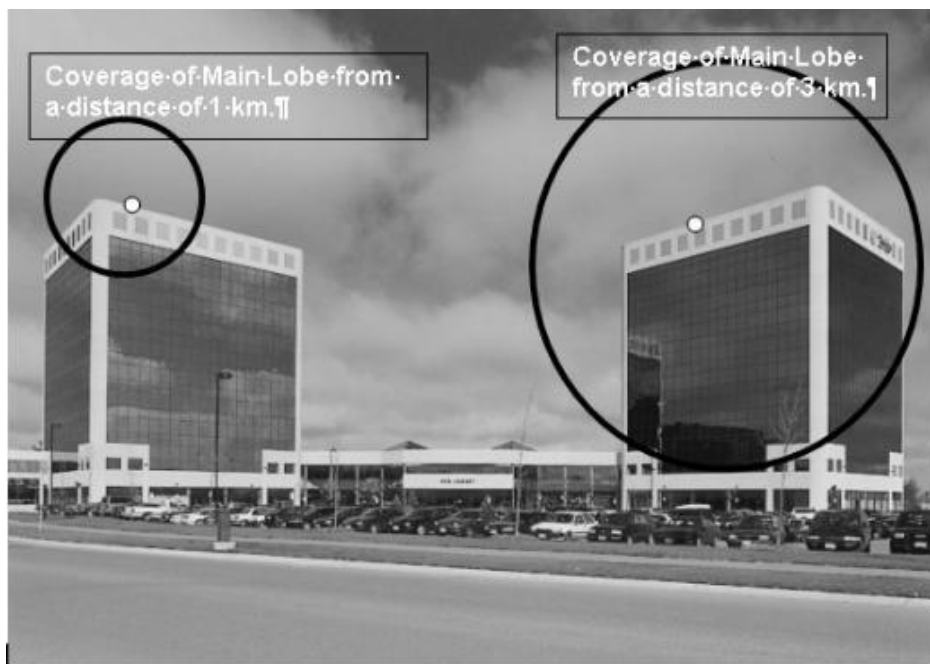
Figure 10-4 Typical main lobe coverage using 23 GHz Radio with 24" dish antenna
