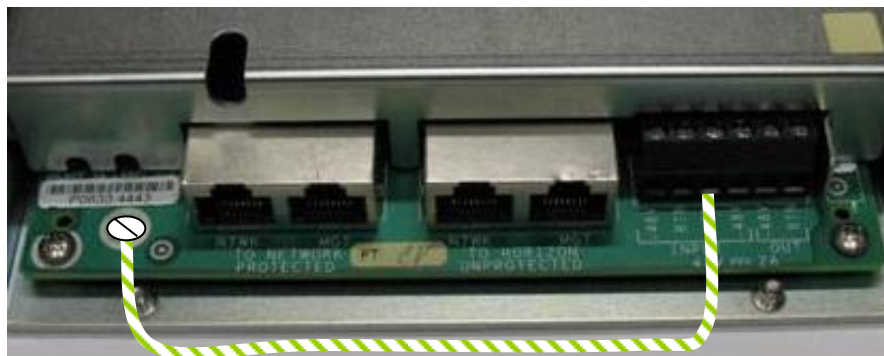
Figure 4-7 Grounded Power Return Shorting Wire
