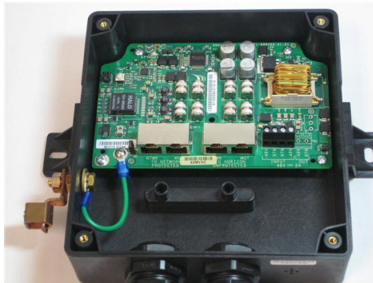
Figure 4-1 Outdoor Lightning Arrestor Unit with Integrated PonE Supply Feed
