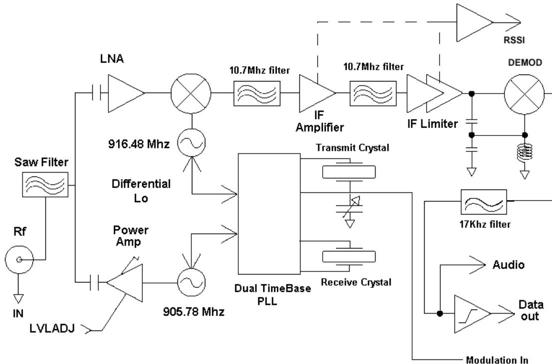
The above block diagram shows the functions blocks of the TR-916-SC transceiver module. On the right side of the diagram the Data out label indicates the point where the RS232 formed data exits the module and is connected to the 15 pin connector at the RX Pin. The Modulation In label indicates where the data to be transmitted enters the module. This is connected to the TX pin of the 15 pin connector. Below is a table list The the inputs and outputs.
