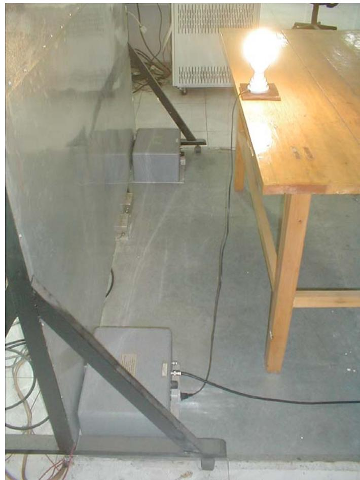
**Photograph of Radiated Emission Test Setup View**
