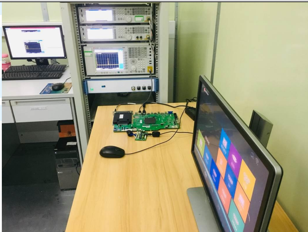
RF Conducted Test Setup
