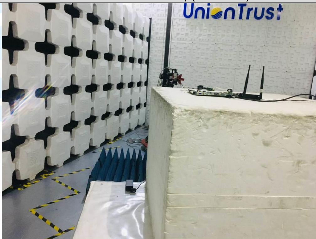
Radiated emission Test Setup (Above 1 GHz)
