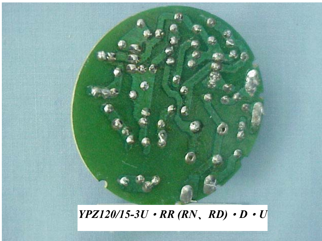
FIGURE 15 SELF-BALLASTED LAMPS FOR GENERAL LIGHTING (M/N: YPZ120/15-3U • RR (RN, RD) • D • U) MAIN BOARD (SOLDERED SIDE)
