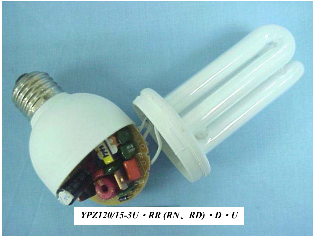
FIGURE 13 SELF-BALLASTED LAMPS FOR GENERAL LIGHTING (M/N: YPZ120/15-3U • RR (RN, RD) • D • U) COVER REMOVED
