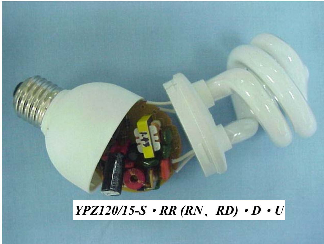
FIGURE 1 SELF-BALLASTED LAMPS FOR GENERAL LIGHTING (M/N: YPZ120/15-S • RR (RN, RD) • D • U) COVER REMOVED
