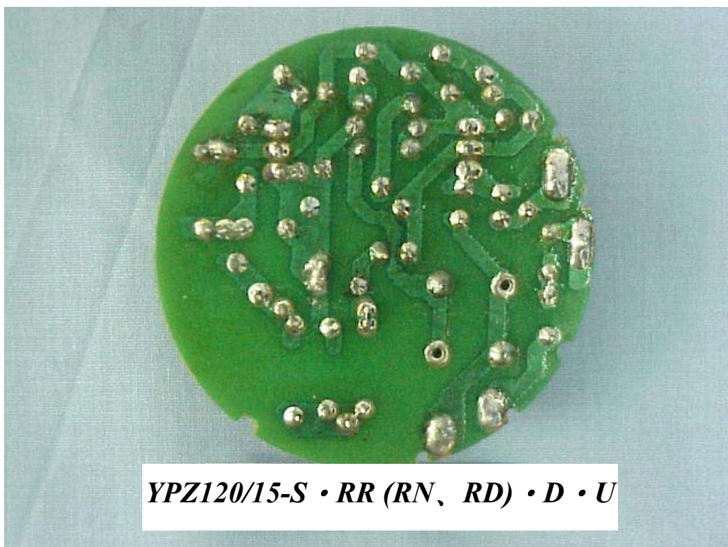
FIGURE 3 SELF-BALLASTED LAMPS FOR GENERAL LIGHTING (M/N: YPZ120/15-S • RR (RN, RD) • D • U) MAIN BOARD (SOLDERED SIDE)
