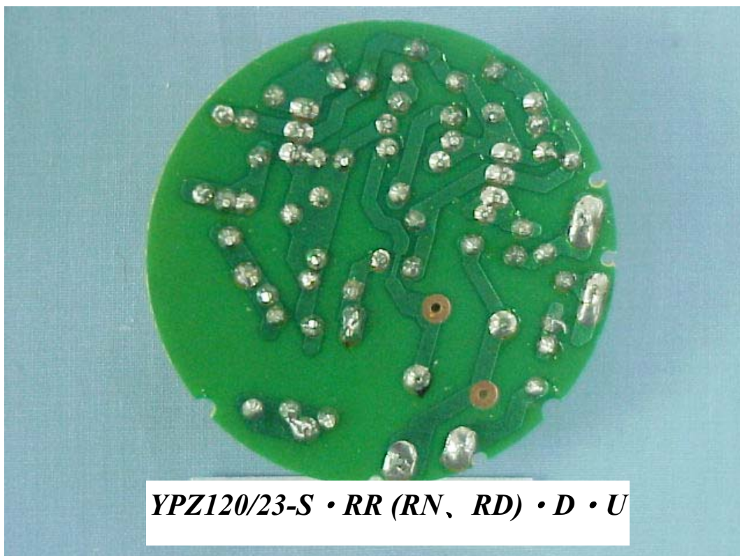
FIGURE 9 SELF-BALLASTED LAMPS FOR GENERAL LIGHTING (M/N: YPZ120/23-S • RR (RN, RD) • D • U) MAIN BOARD (SOLDERED SIDE)
