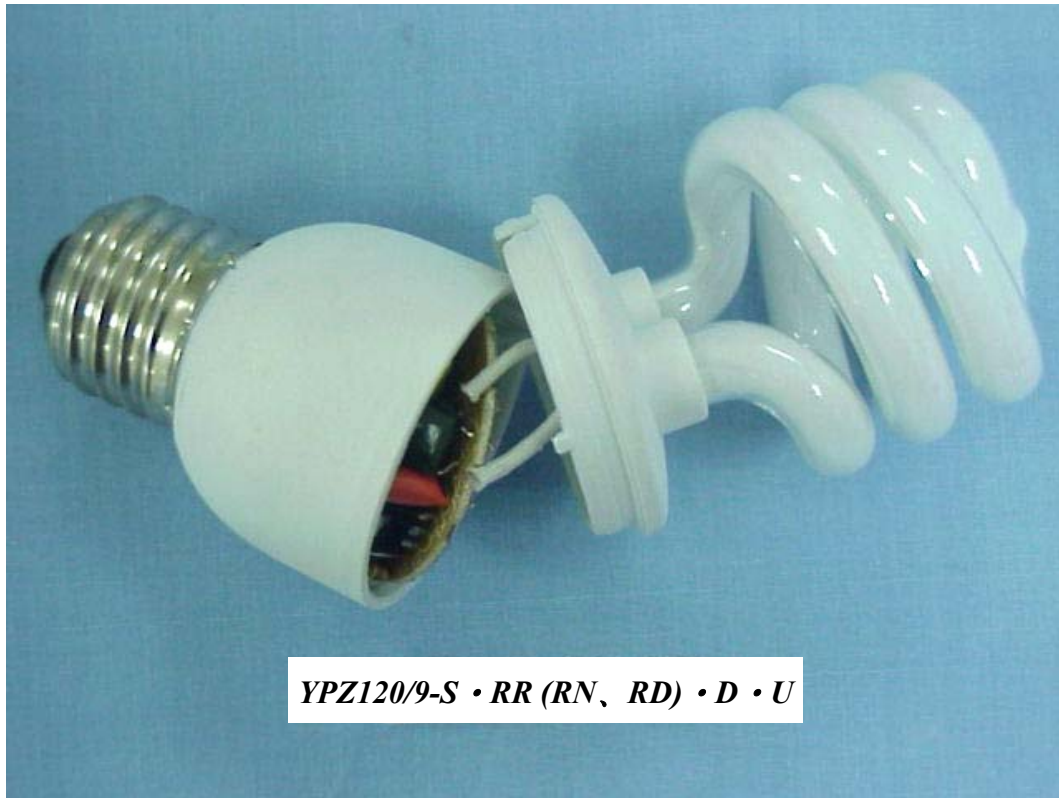
FIGURE 1 SELF-BALLASTED LAMPS FOR GENERAL LIGHTING (M/N: YPZ120/9-S • RR (RN, RD) • D • U) COVER REMOVED
