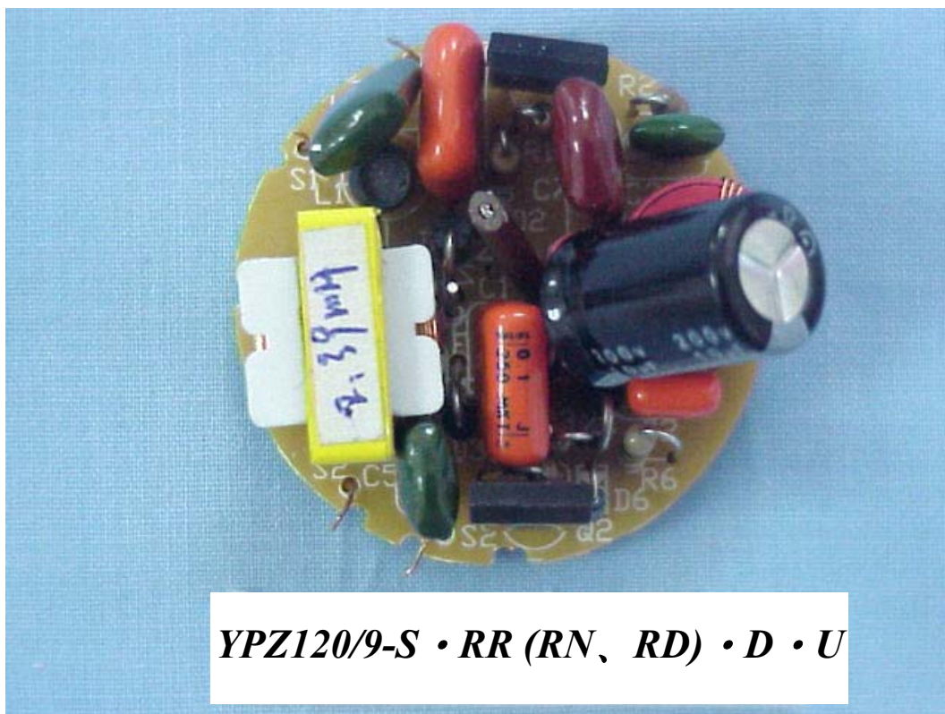
FIGURE 2 SELF-BALLASTED LAMPS FOR GENERAL LIGHTING (M/N: YPZ120/9-S • RR (RN, RD) • D • U) MAIN BOARD (COMPONENT SIDE)
