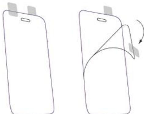
2. Separate about half of the release film layer and start applying the Steinheil™ Ultra film on to the device. Remove the rest of the release film layer as you install it. Slightly sweep through the surface of the film with the provided squeegee to avoid air bubbles.
