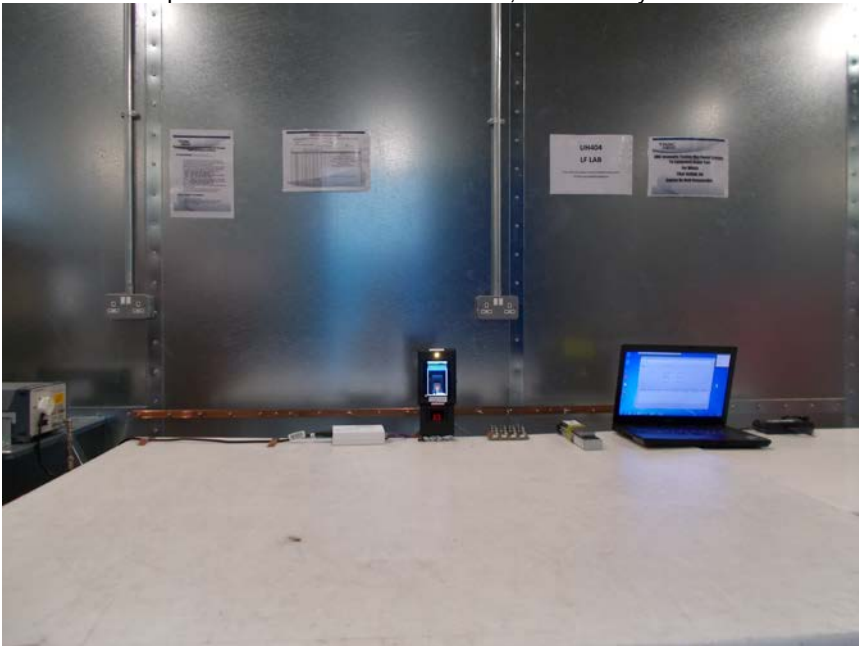
AC power-line conducted emissions, Powered by POE
