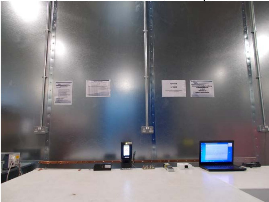
AC power-line conducted emissions, Powered by POE
