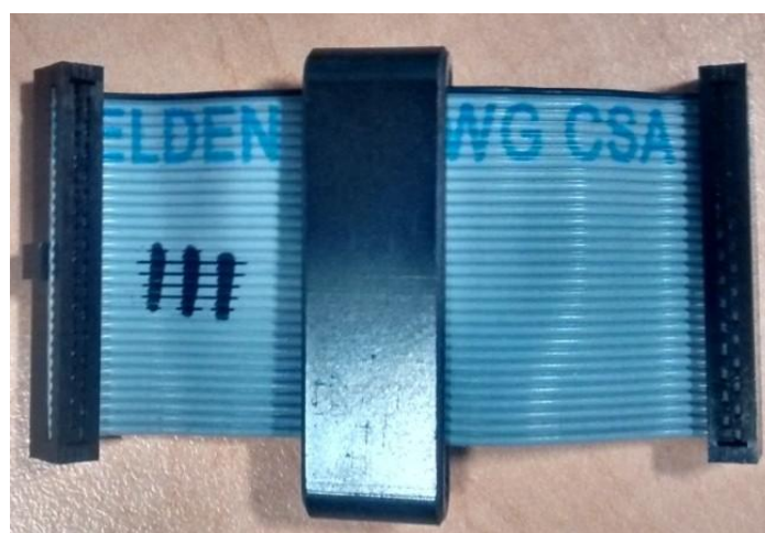
Cable - INT-CON-RIB-ASSY, Rev 3 Connects between Main PCB and I/O PCB
