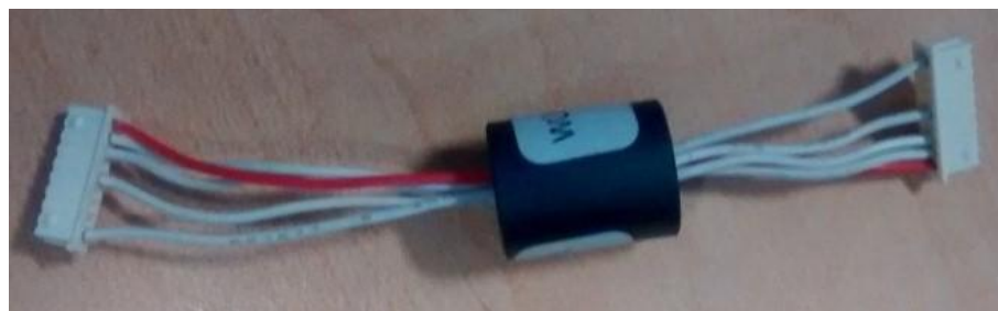
Cable - Suprema-711-Assy, Rev 2 Connects between BIO cable assy's PCB and the Suprema PCB
