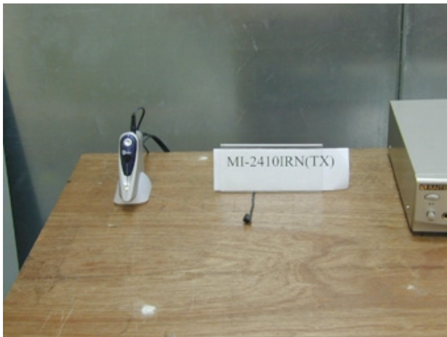
Photo 2: Conducted Test Set-up (enlarge)
