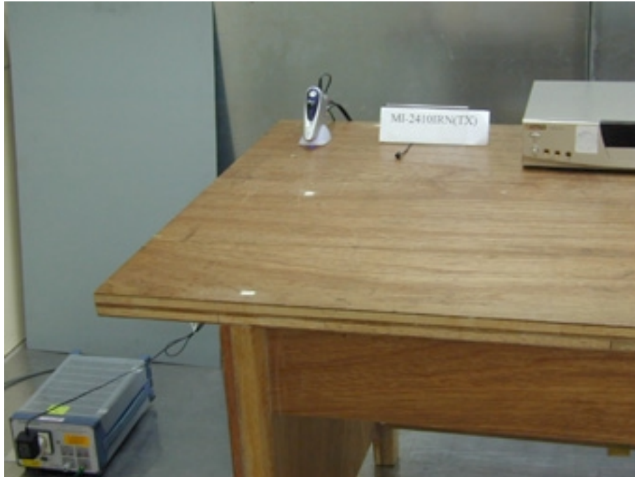
Photo 1: Conducted Test Set-up (front view)
