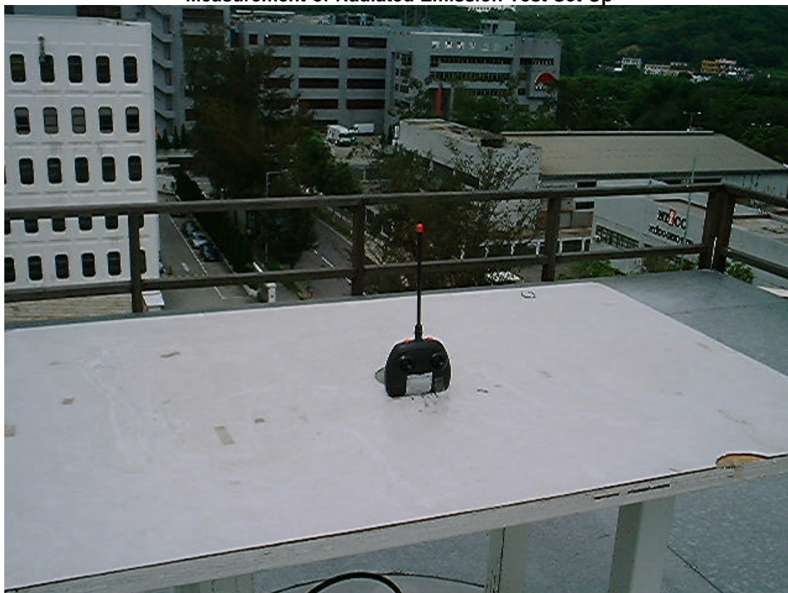
Measurement of Radiated Emission Test Set Up
