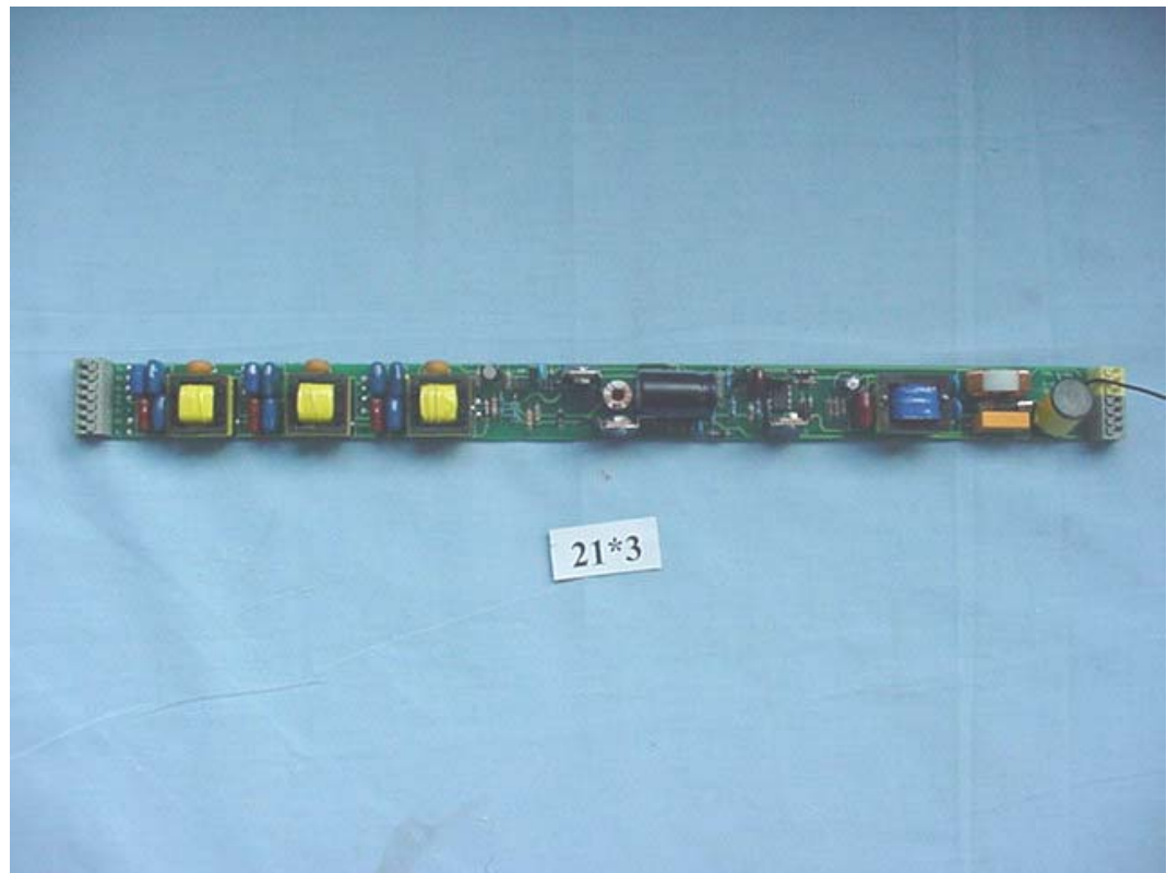
FIGURE 5 BALLAST (M/N: FBT T5 21x3) MAIN BOARD (COMPONENT SIDE)
