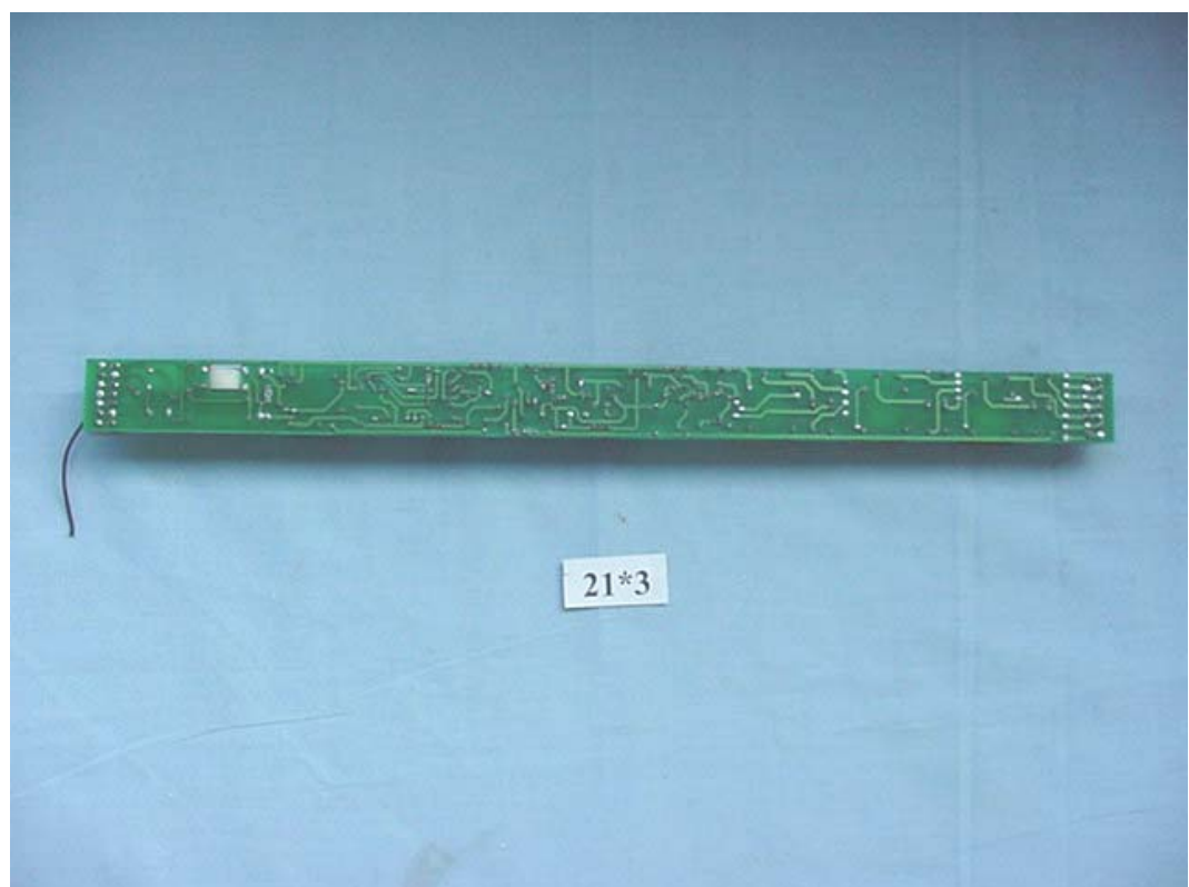
FIGURE 6 BALLAST (M/N: FBT T5 21x3) MAIN BOARD (SOLDERED SIDE)
