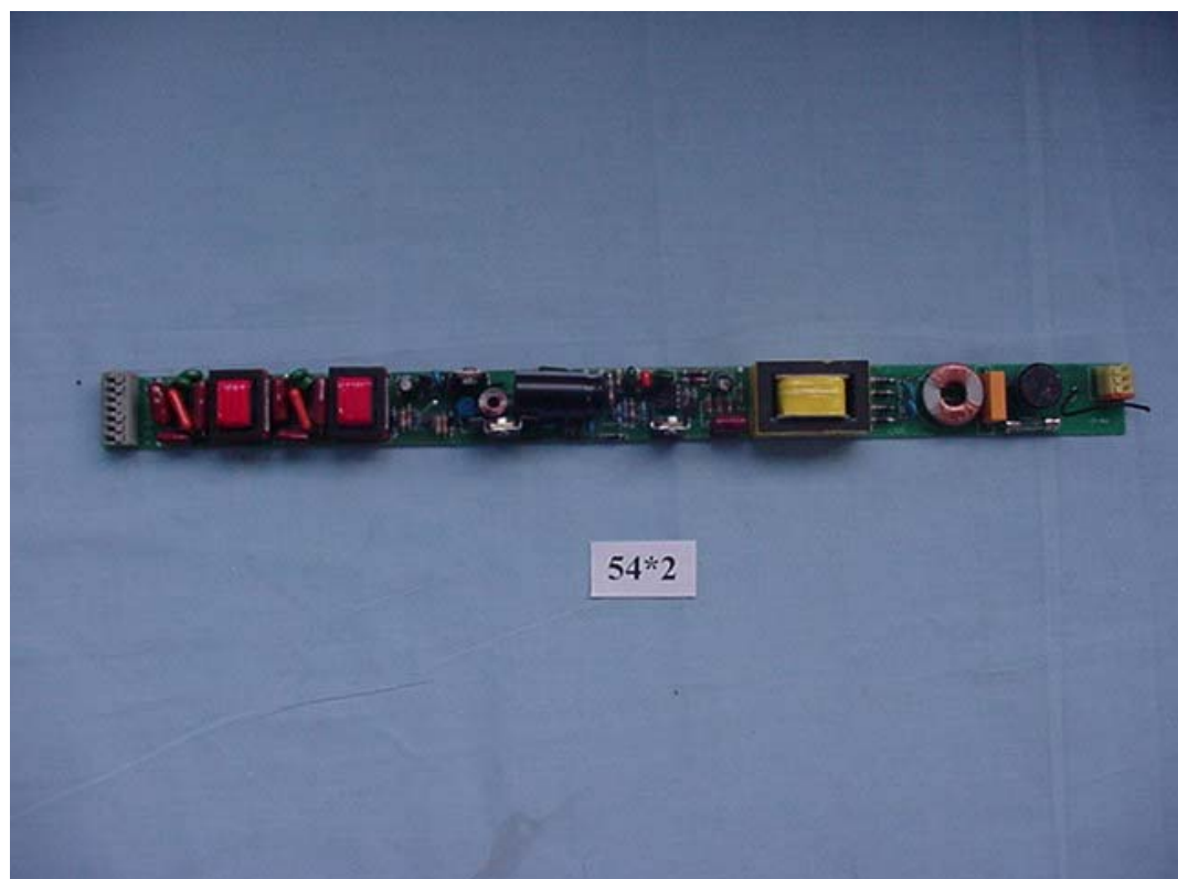
FIGURE 14 BALLAST (M/N: FBT T5 54X2) MAIN BOARD (COMPONENT SIDE)
