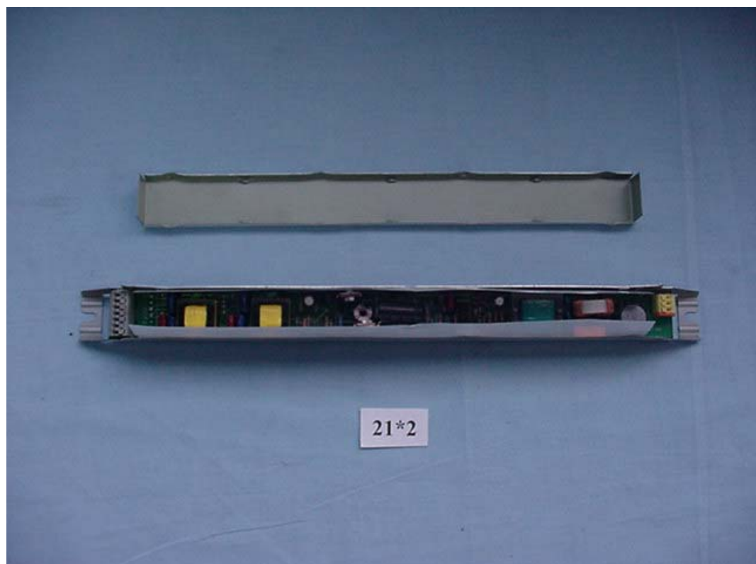
FIGURE 4 BALLAST (M/N: FBT T5 21X2) COVER REMOVED
