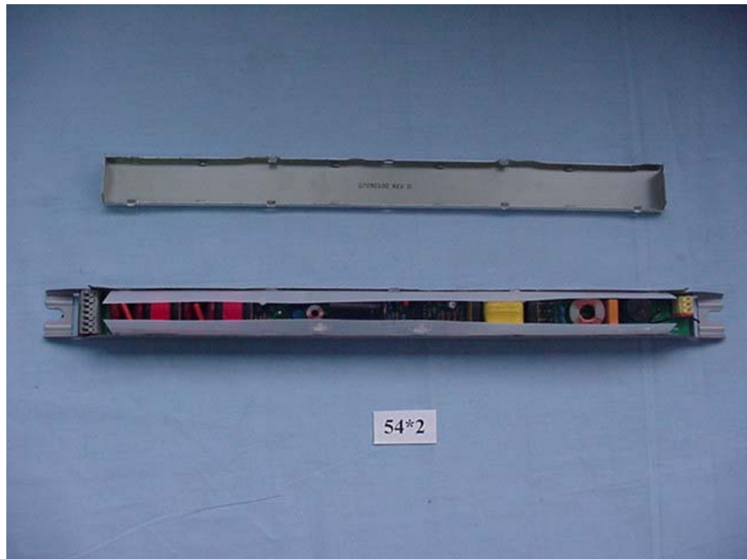
Figure 13 BALLAST (M/N: FBT T5 54X2) COVER REMOVED
