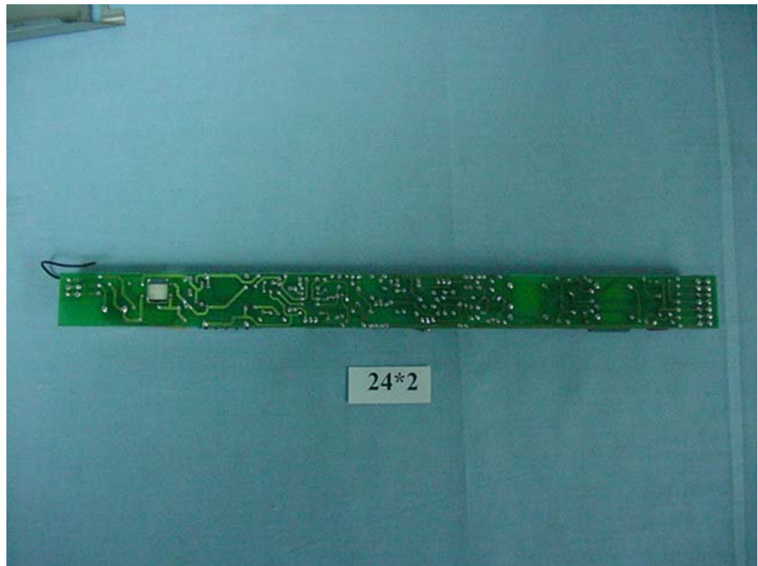
FIGURE 9 BALLAST (M/N: FBT T5 24X2) MAIN BOARD (SOLDERED SIDE)
