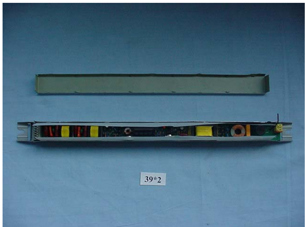
FIGURE 10 BALLAST (M/N: FBT T5 39X2) COVER REMOVED
