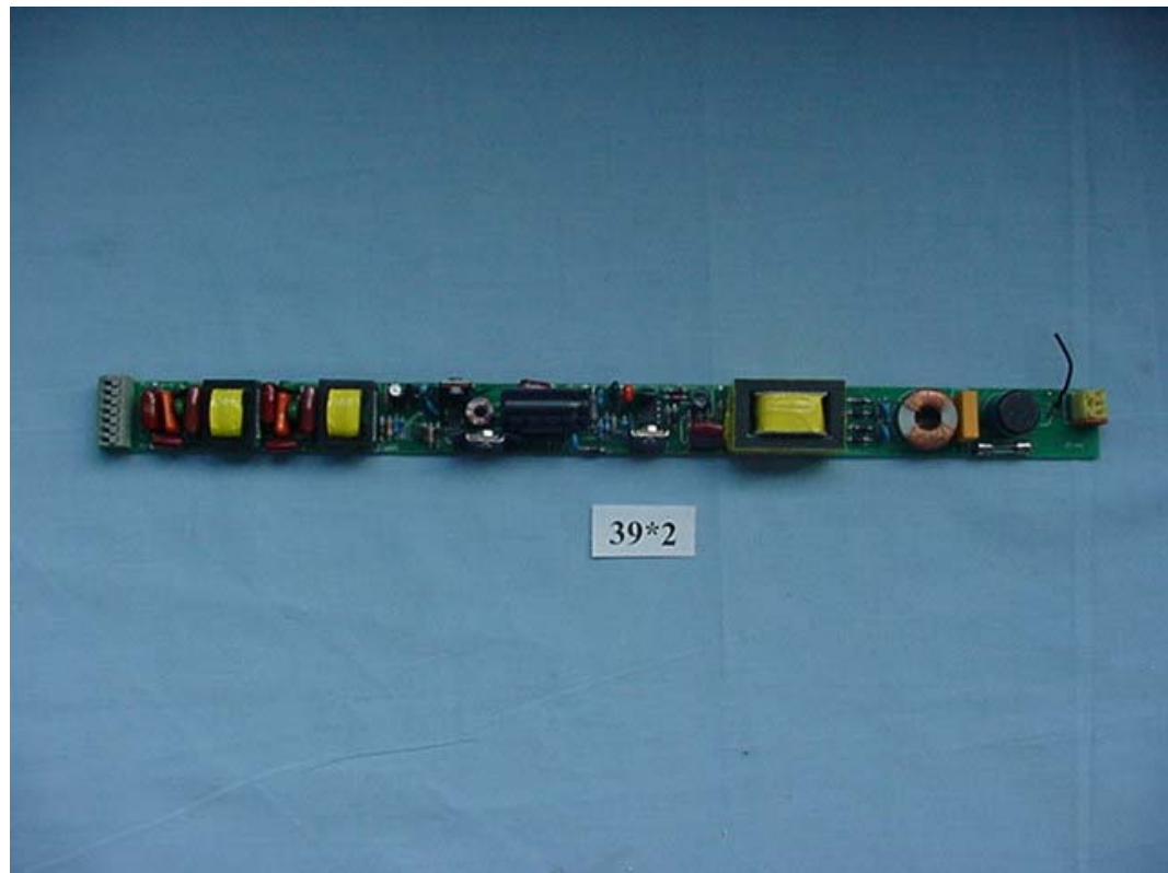
FIGURE 11 BALLAST (M/N: FBT T5 39X2) MAIN BOARD (COMPONENT SIDE)
