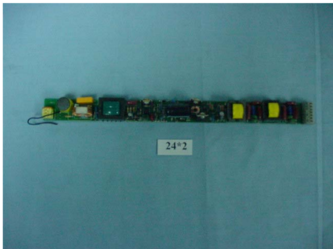
FIGURE 8 BALLAST (M/N: FBT T5 24X2) MAIN BOARD (COMPONENT SIDE)
