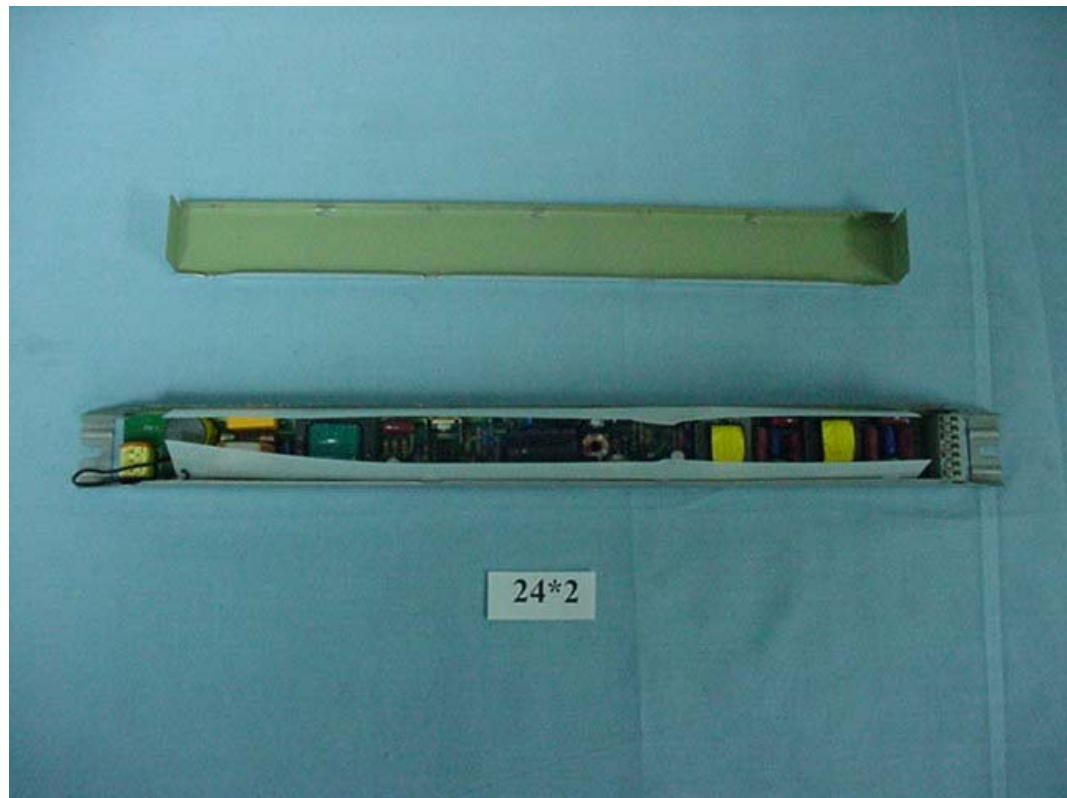
FIGURE 7 BALLAST (M/N: FBT T5 24X2) COVER REMOVED
