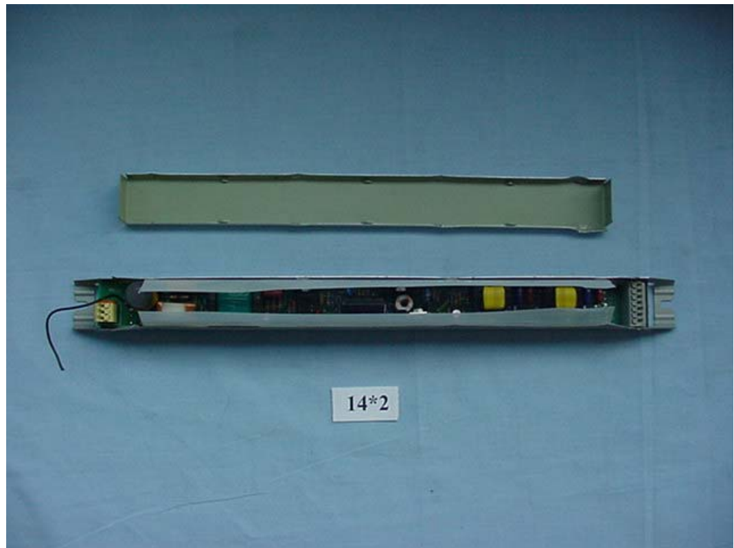
FIGURE 1 BALLAST (M/N: FBT T5 14X2) COVER REMOVED
