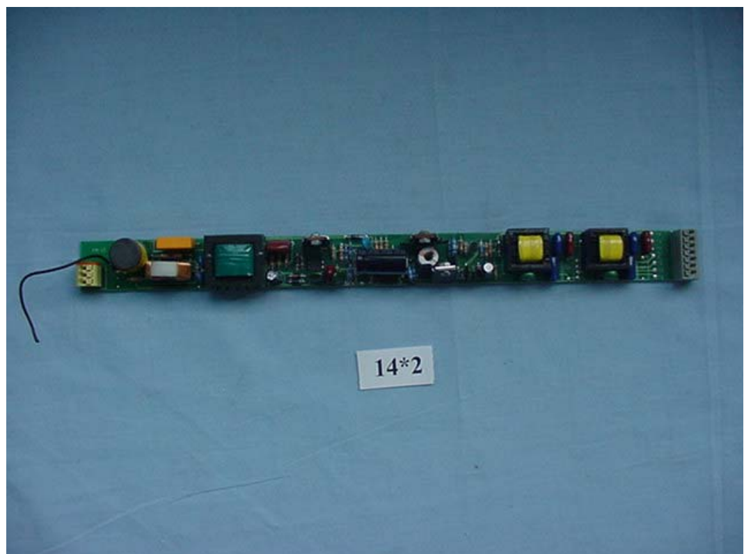
FIGURE 2 BALLAST (M/N: FBT T5 14X2) MAIN BOARD (COMPONENT SIDE)
