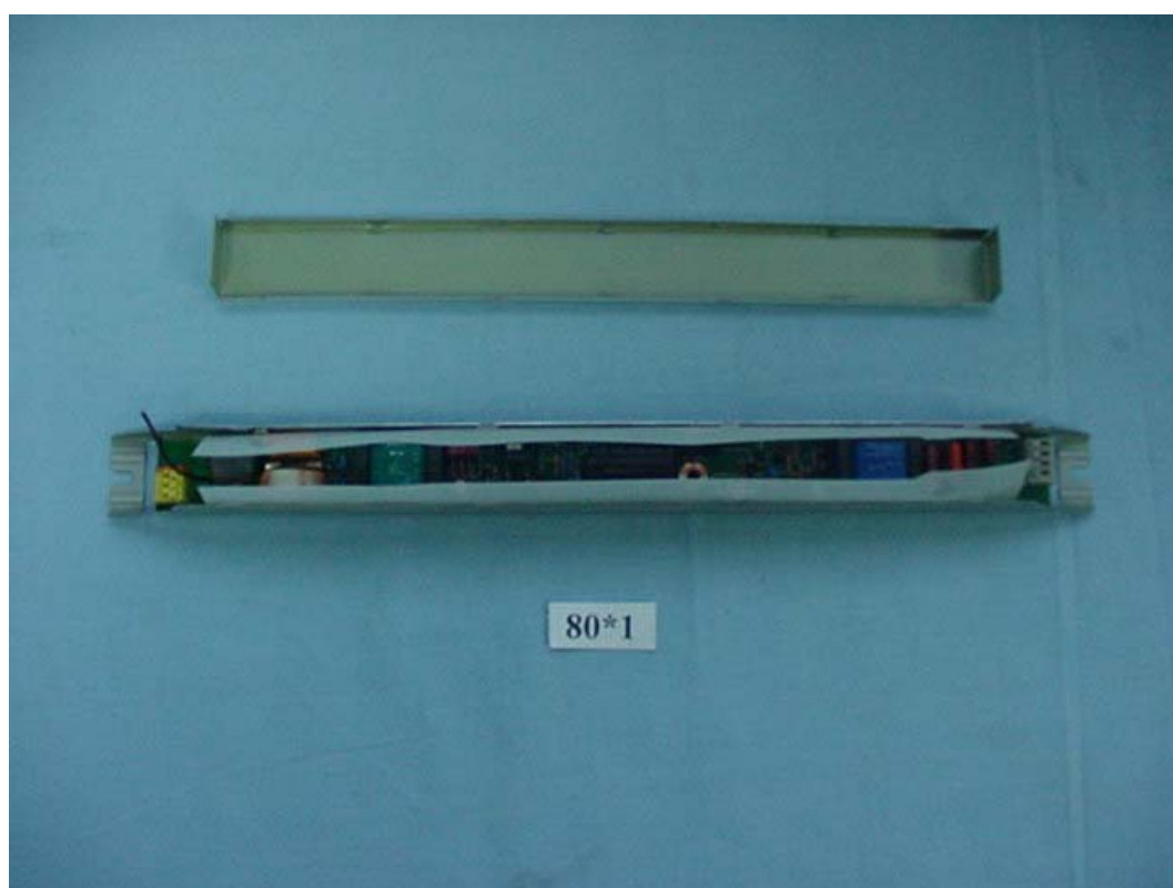
FIGURE 16 BALLAST (M/N: FBT T5 80x1) COVER REMOVED
