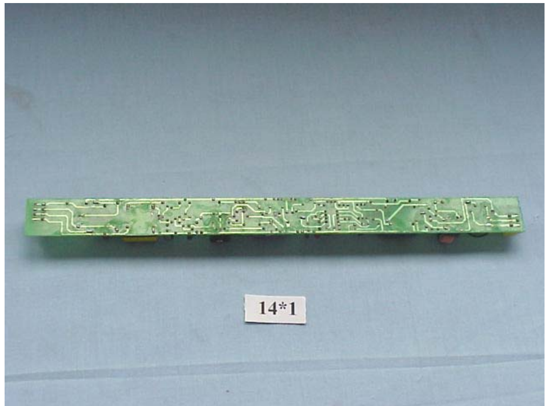
FIGURE 3 BALLAST (M/N: FBT T5 14x1) MAIN BOARD (SOLDERED SIDE)
