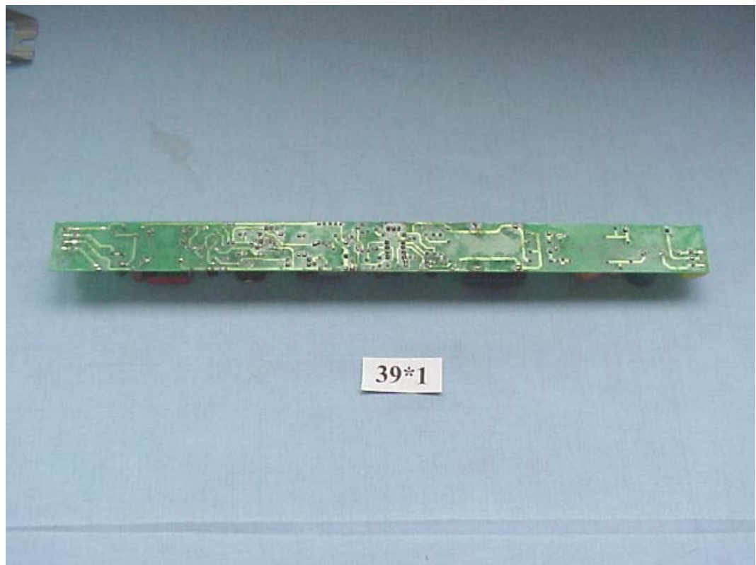
FIGURE 12 BALLAST (M/N: FBT T5 39X1) MAIN BOARD (SOLDERED SIDE)
