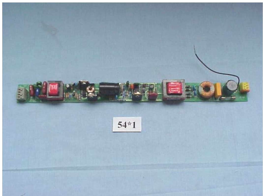
FIGURE 14 BALLAST (M/N: FBT T5 54x1) MAIN BOARD (COMPONENT SIDE)
