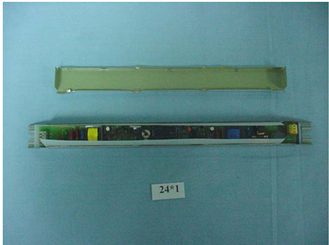
FIGURE 7 BALLAST (M/N: FBT T5 24x1) COVER REMOVED
