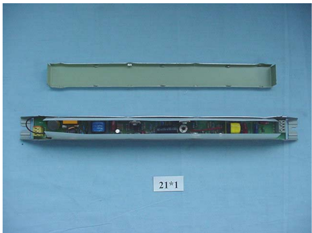
FIGURE 4 BALLAST (M/N: FBT T5 21x1) COVER REMOVED
