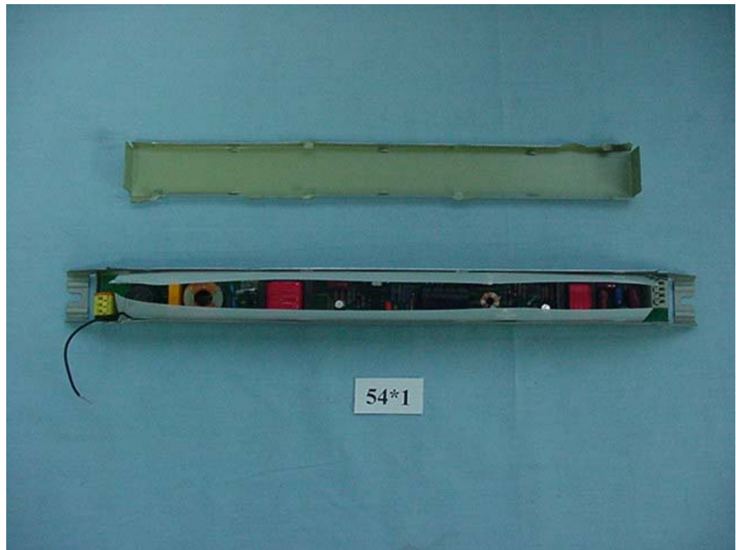
Figure 13 BALLAST (M/N: FBT T5 54x1) COVER REMOVED
