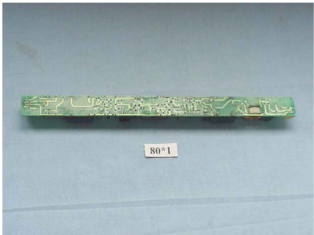
FIGURE 18 BALLAST (M/N: FBT T5 80X1) MAIN BOARD (SOLDERED SIDE)
