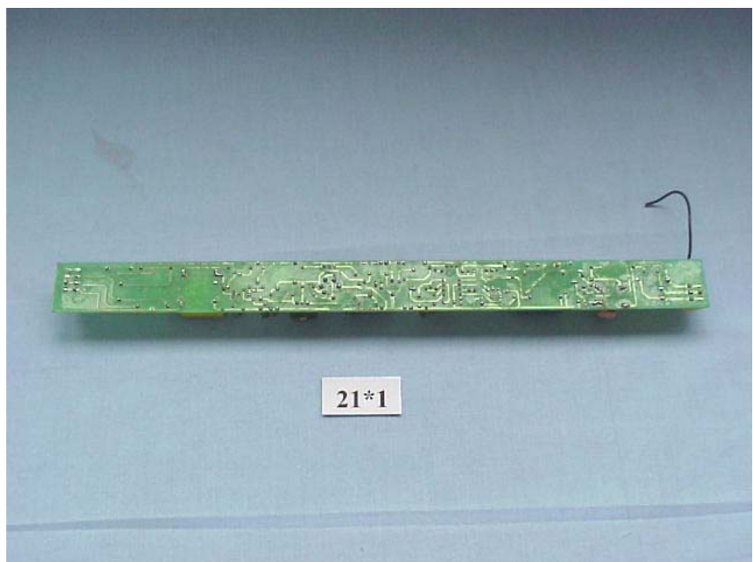
FIGURE 6 BALLAST (M/N: FBT T5 21x1) MAIN BOARD (SOLDERED SIDE)
