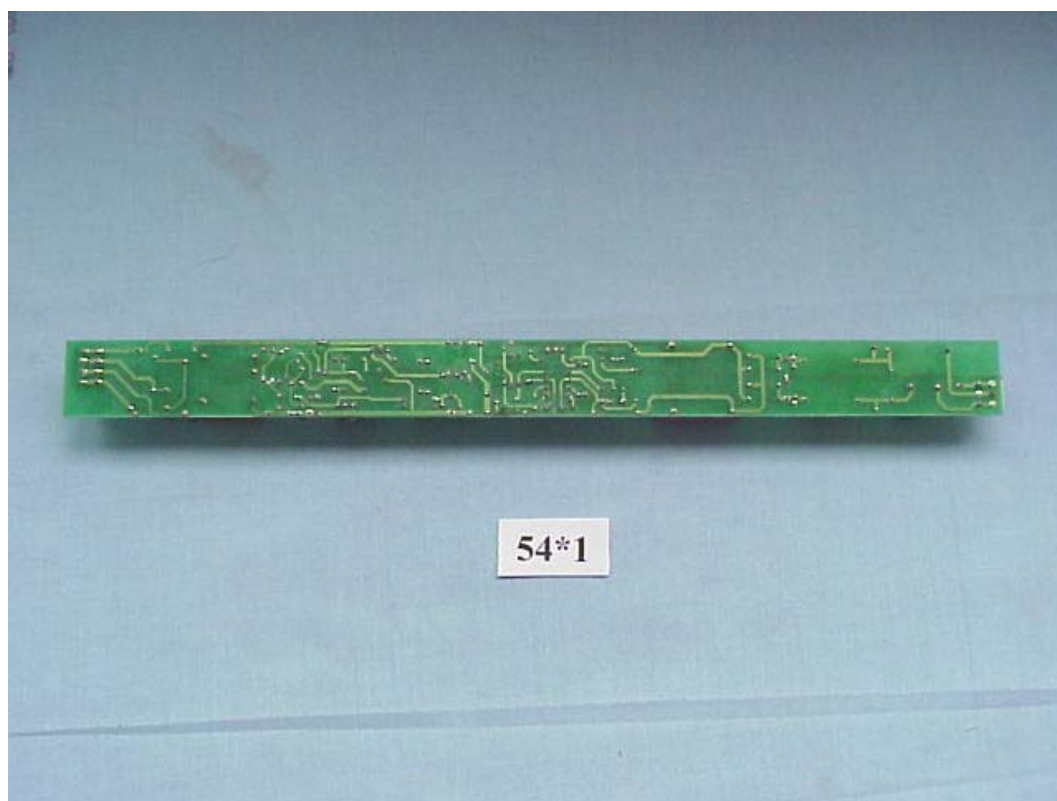
FIGURE 15 BALLAST (M/N: FBT T5 54x1) MAIN BOARD (SOLDERED SIDE)
