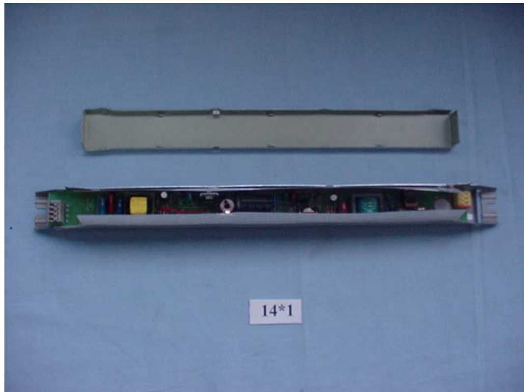
FIGURE 1 BALLAST (M/N: FBT T5 14x1) COVER REMOVED
