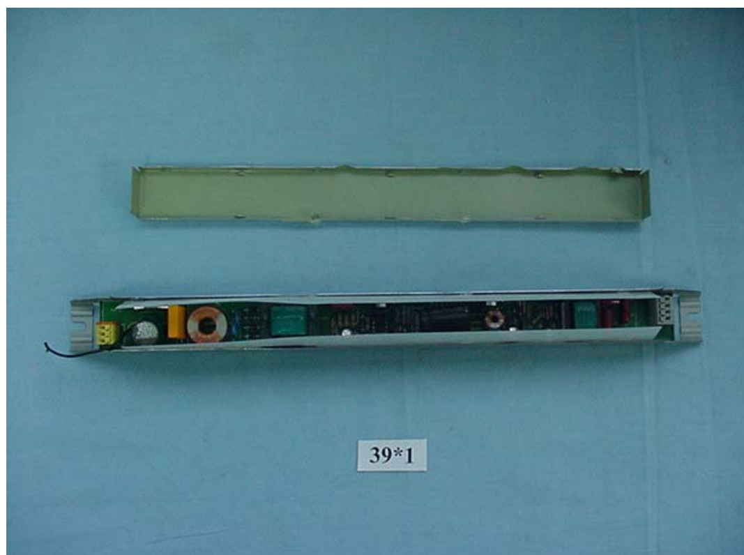
FIGURE 10 BALLAST (M/N: FBT T5 39x1) COVER REMOVED
