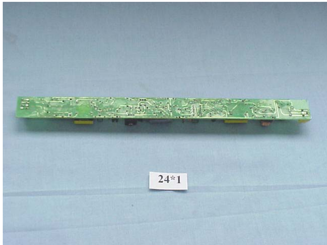
FIGURE 9 BALLAST (M/N: FBT T5 24x1) MAIN BOARD (SOLDERED SIDE)
