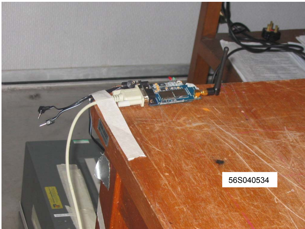
Conducted Emissions Setup (Rear View)
