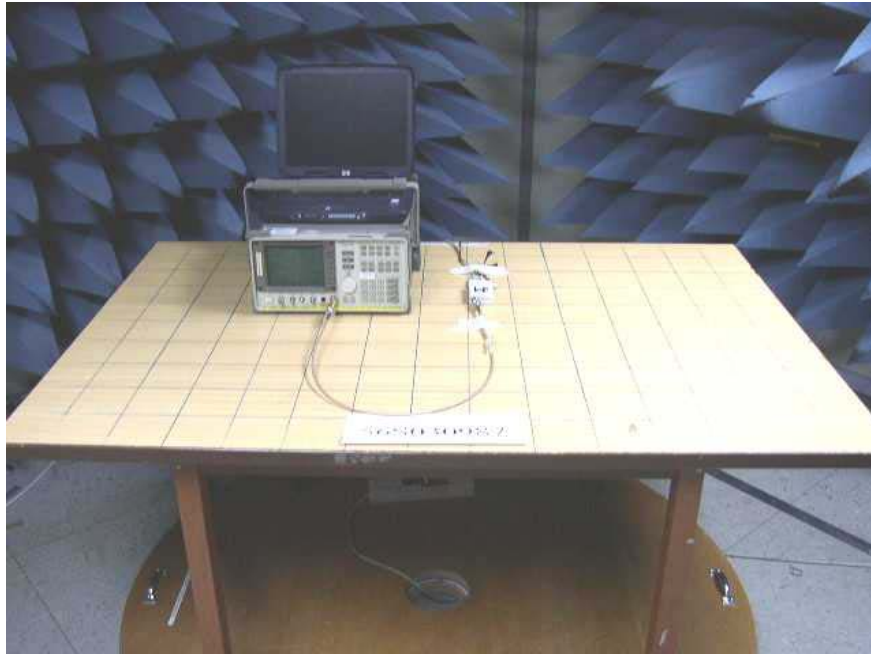
Number of Hopping Frequencies Measurement Test Setup
