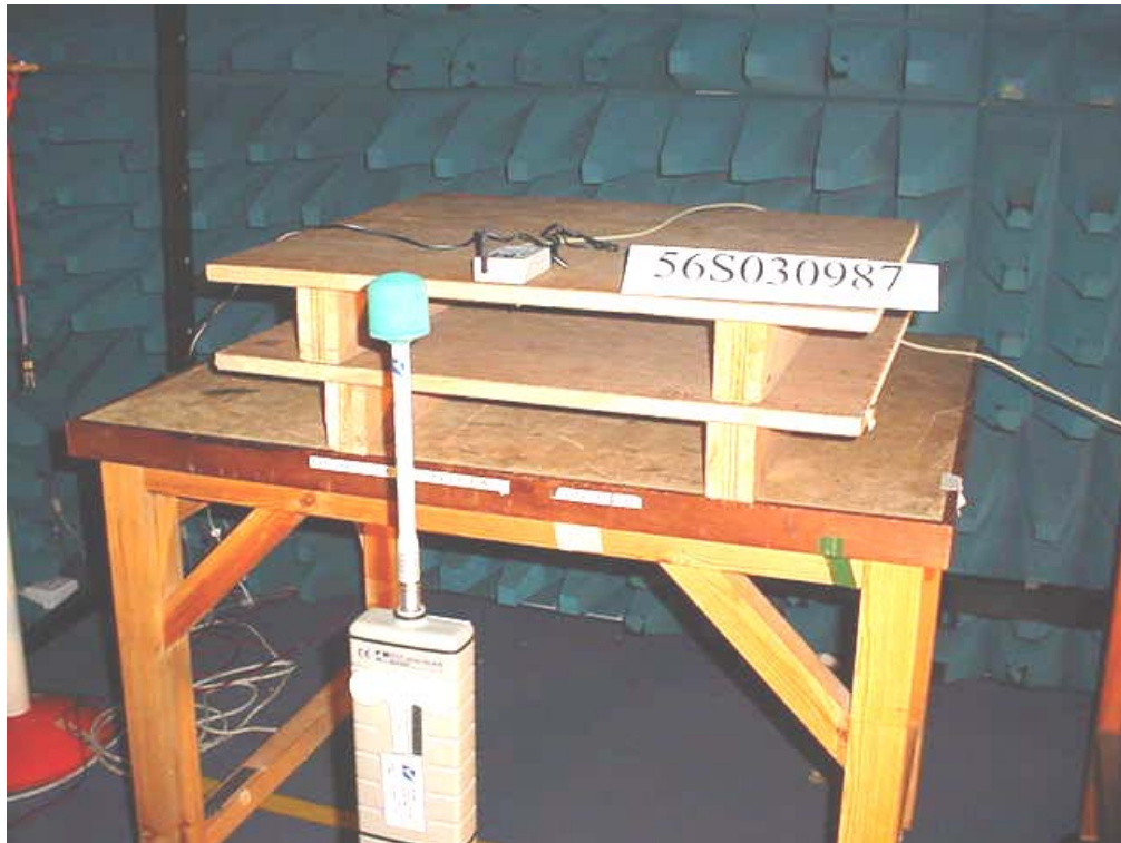
Maximum Permissible Exposure Measurement Test Setup
