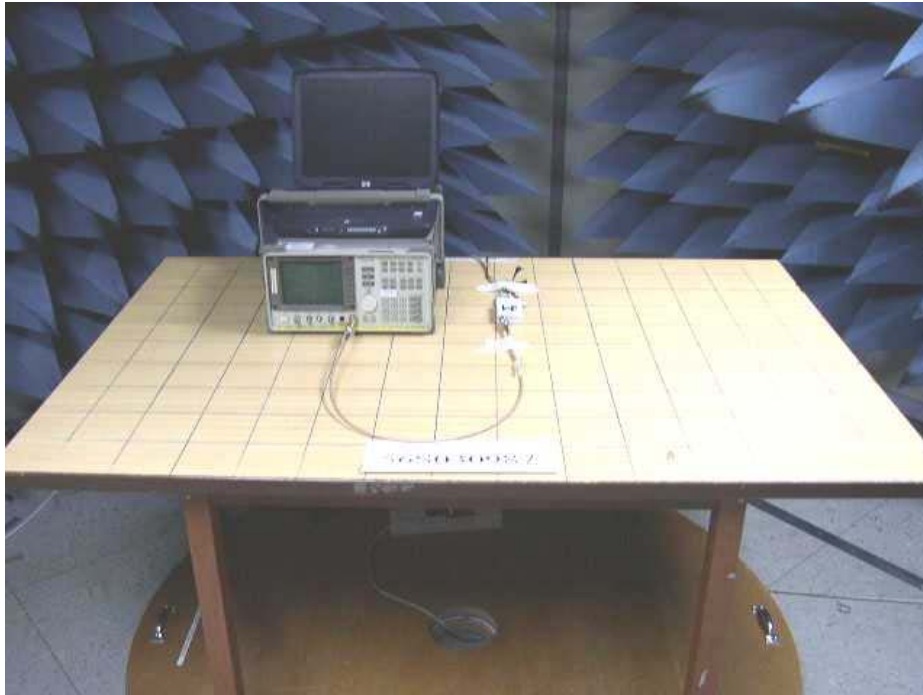
Number of Hopping Frequencies Measurement Test Setup
