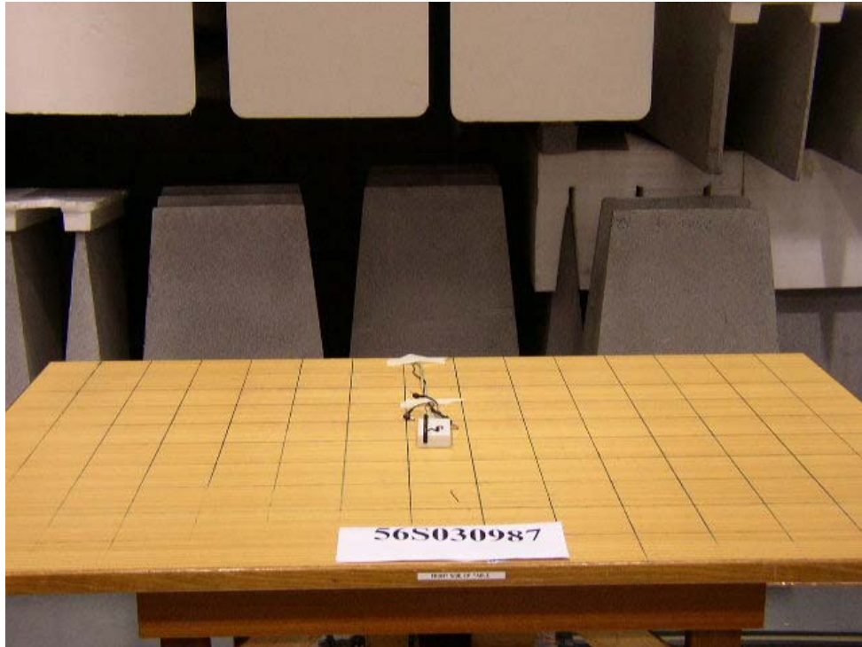
Radiated Emissions Setup (Front View)
