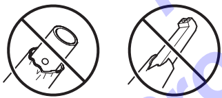
Figure 108 – Tip Sleeve Damage
