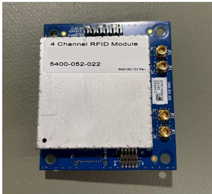
Figure 7. RF Module PCBA Top View with cover
