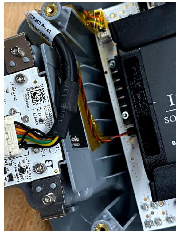
NFC Antenna Mounted and Connected to PCBA
