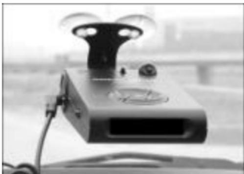
Slide the detector onto the bracket and get it locked with switch.
