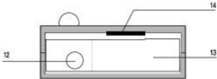
12. Laser Lens (Front) High gain optical lens array provides increased sensitivity and field of view for leading edge laser detection.
