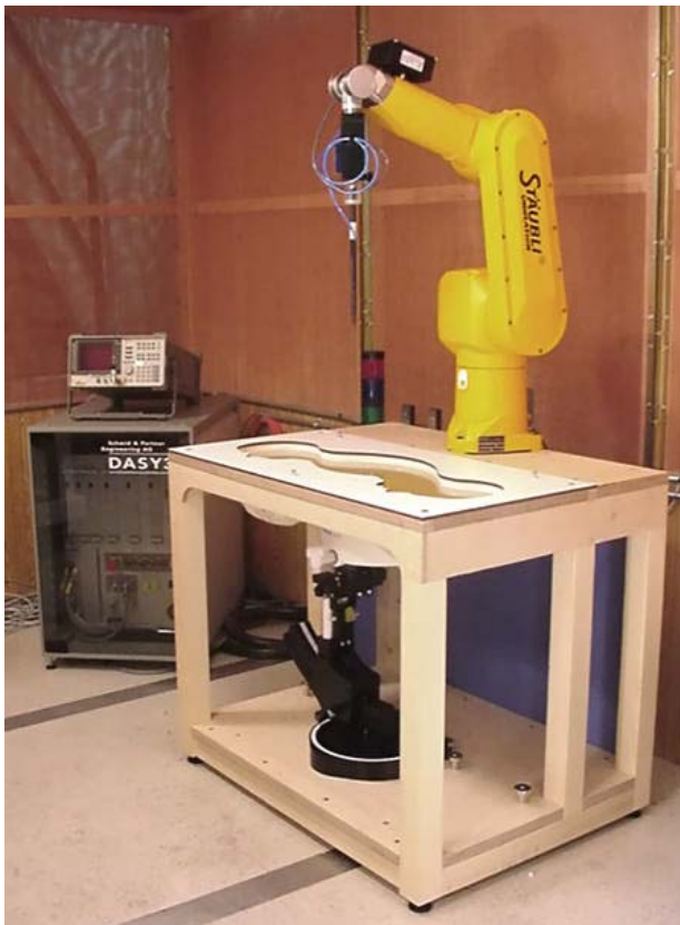
DASY3 SAR Measurement System with SAM Phantom
