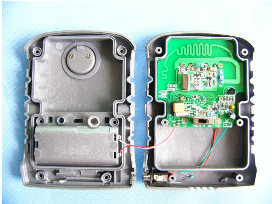
(4) Main board component side
