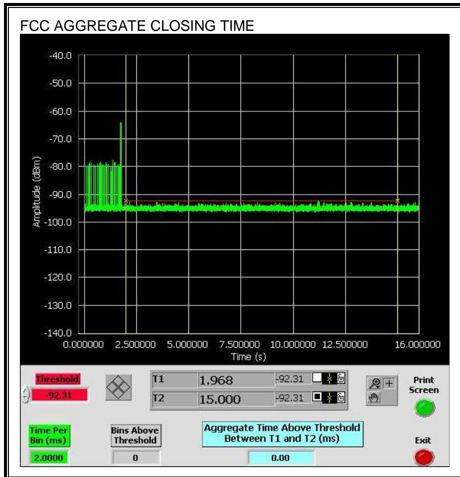
No transmissions are observed during the IC aggregate monitoring period.
