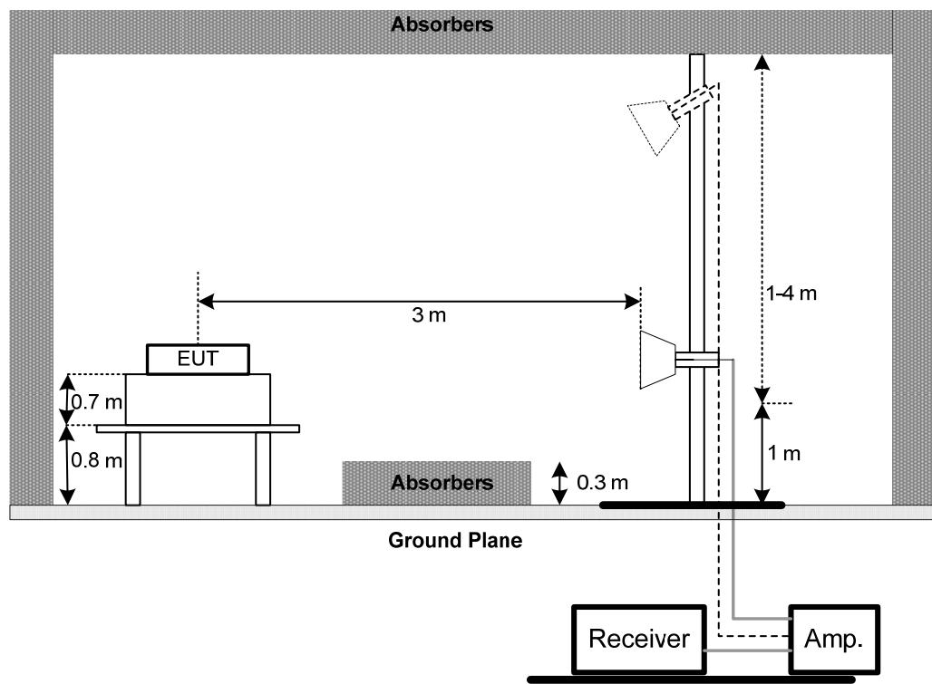
(C) For radiated emissions below 30MHz
