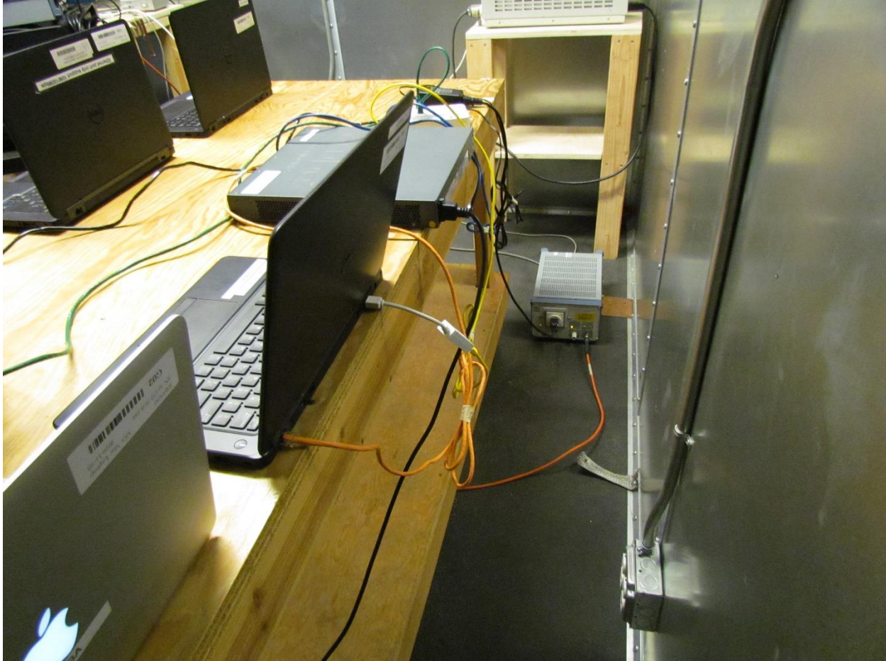
Conducted Emissions ACDC config Rear View
