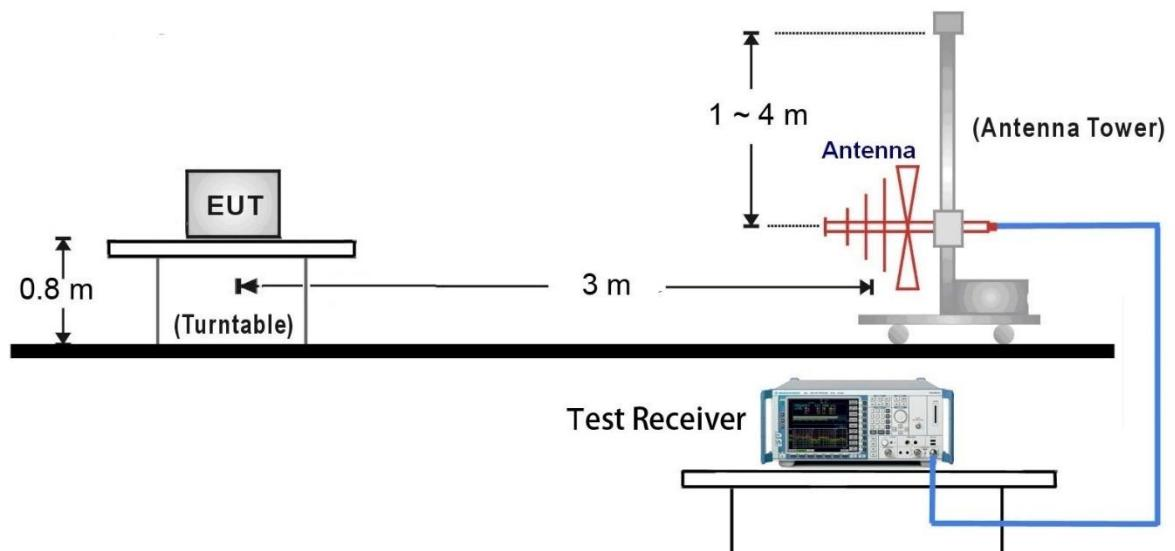
1GHz ~ 25GHz Test Setup:
