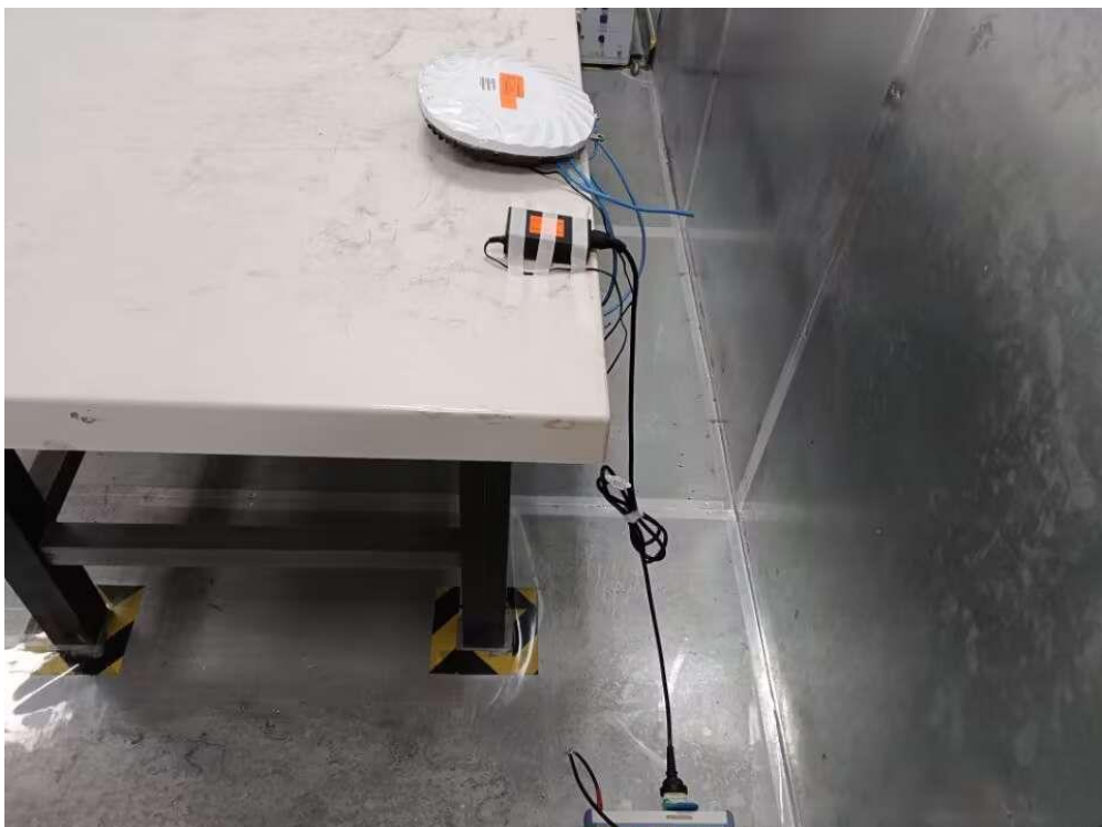
Description: Test Setup for Conducted Emissions
