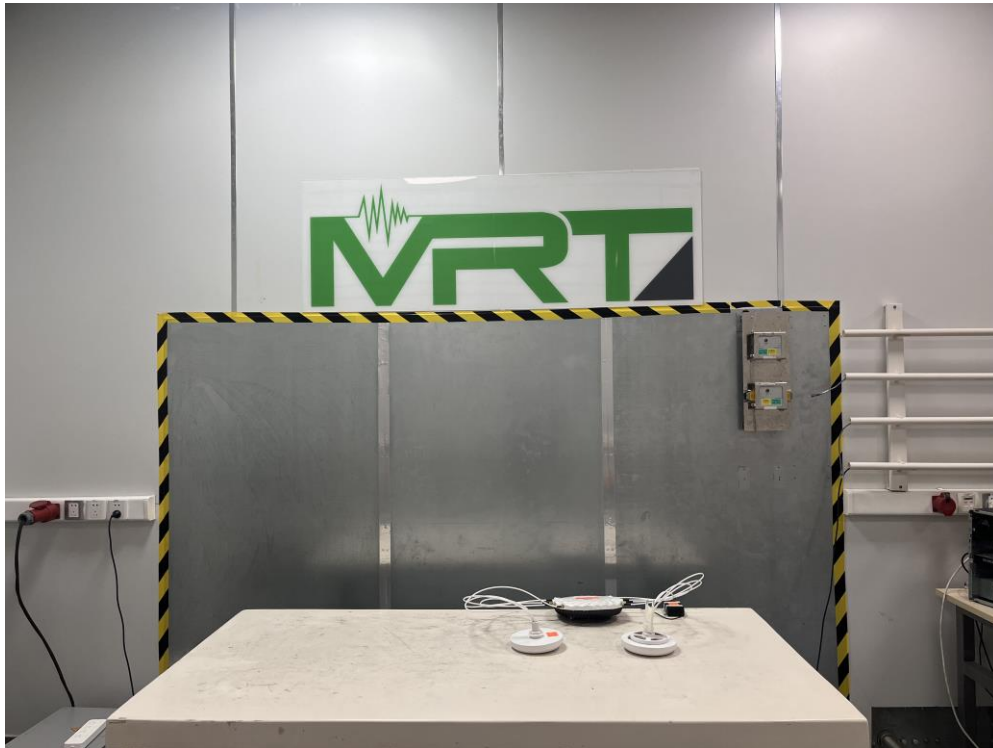
Description: Test Setup for Conducted Emissions
