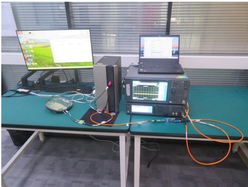
Description: DFS Test Setup
