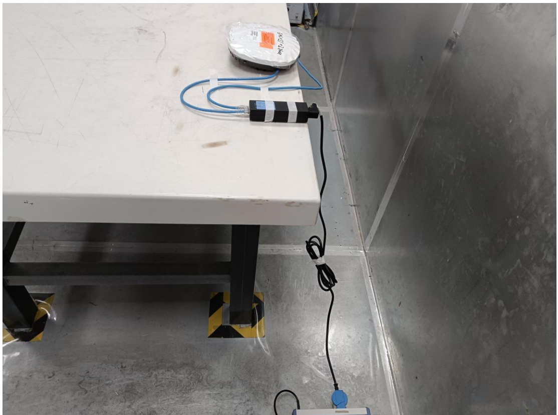
Description: Conducted Emission – Side View
