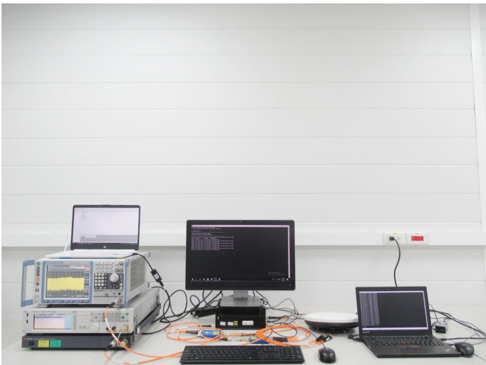
Description: DFS Test Setup _ Conducted
