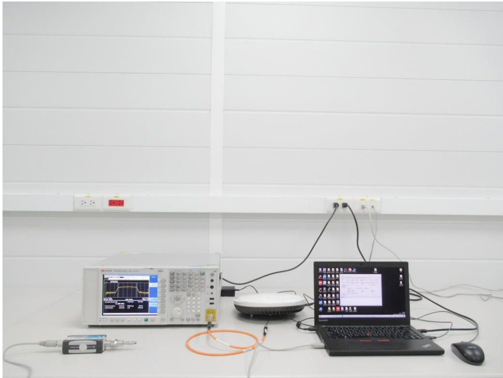
Description: DFS Test Setup _ Conducted
