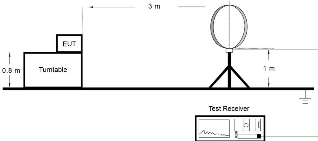
Below 1GHz Test Setup:
